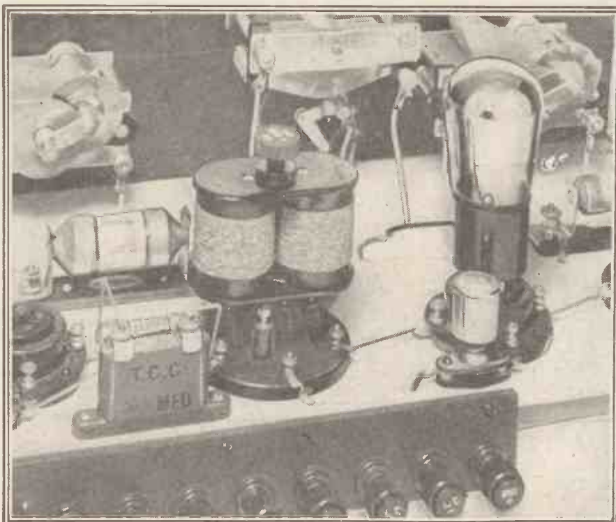
If an ordinary valve were employed in this receiver, a neutralising condenser would be needed. But with the "Interdyne" the extra connection serves the same purpose.
