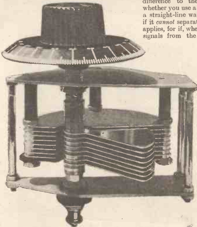
One type of square-law condenser, without vernier dial.
