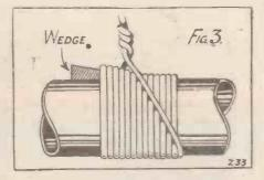
permissible, a direct earth outside the house is usually rather better than the water-pipe earth, but the main factor governing the final decision is the resulting length of the earth lead, and a personal test is the surest way of getting the best answer. If recourse is made to the water pipe, pay attention to the following points.
