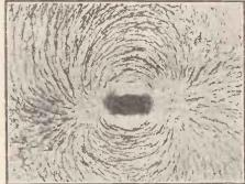
Fig. 2. Showing the field of magnetic force existing around the poles of an efficient headphone magnet.
