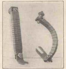
Fig. 5. Two forms of home-made resistors.
