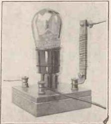
The resistor in place on the filament terminal of the valve holder.
