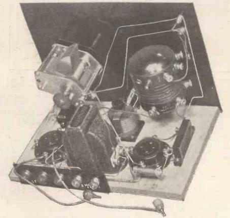
As the back of panel shows the grid leak is soldered directly into circuit. Two small clips could be used and there would be room to mount the component on the baseboard,
