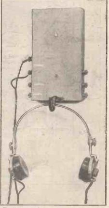
The "Stethocrys" is not merely an automatically aerial-earthing set. The simple action of hanging up or taking off 'phones does much more than this.
