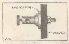
green on the negative. Next you will have to screw the terminals to the panel by means of the nuts, as shown in the sketch. These counters are likely to be made of bone, and thus prove to be excellent insulators for a wood panel if one is placed at each side of the panel.
