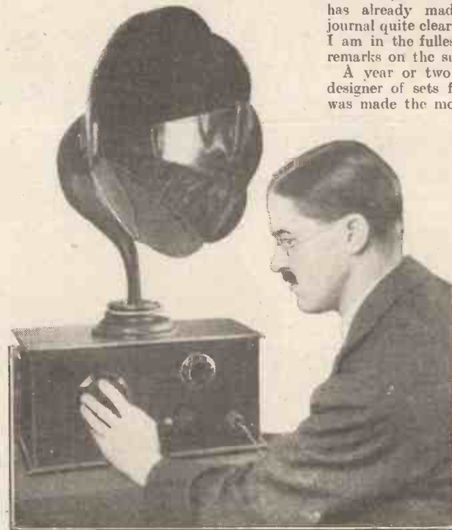
Operating the one-valve loud speaker set described in this issue.
