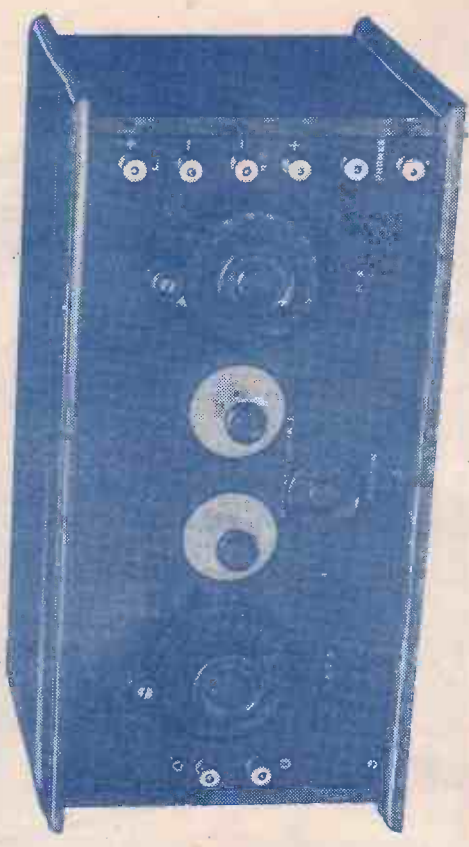
The complete two-valve receiver. Note the convenient positions of the various controls. This is not a difficult task, especially if the constructor is more or less used to the operation of soldering. If he is not so used, we advise him to try it, because a well soldered set is, in our opinion, far more satisfactory, both in appearance and operation, than one in which the connections have been made
