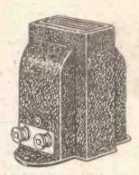
GECOPHONE L.F. CHOKE is a neat and compact com-ponent for use in choke-coupled L.F. stages. High value of inductance gives maximum amplification of the lower frequencies and ensures natural reproduction. The new circuit uses a butt joint to render the inductance more constant.
