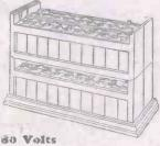
Two tiers of two units each are required. The same base and lid are used as for 40 volts.
