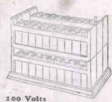
Two tiers are used—the bottom one containing 3 units and the upper one containing only two units with blank end pieces to separate them. For 120 volts the end pieces are removed and a complete unit is substituted.
