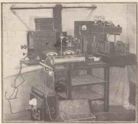
The receiving section of "Mihá'y's experimental television apparatus.
