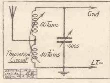
without altering the existing lay-out, a variometer was made in which the 40 turns became the rotor and the 60 turns the stator; the '0005 variable condenser was, of course, still used. In this form it gave very good results and well repaid the time and material used in making it. Should a two-coil holder be used, the wiring should be arranged so that the direction of the coils is the same.
