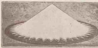
Fig. 4. The paper cone after it has been fixed in position on the frame.
