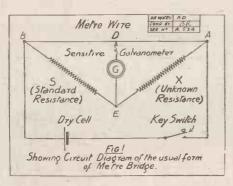
As usually employed, this instrument involves the use of a delicate galvanometer, sensitive to currents of 1 micro-ampere, also a set of standard resistances. It is possible to dispense with the galvanometer, using instead a pair of headphones, which are just as sensitive; and if one or two standard resistances are purchased the rest of the set can easily be made. The instrument itself is also easy and cheap to make.
