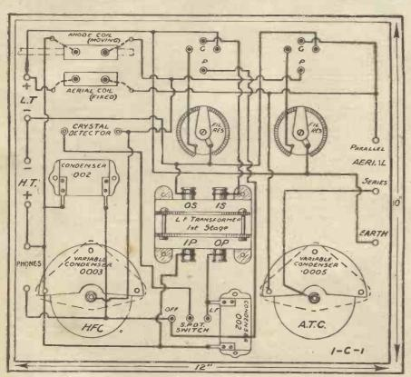
terminal, and the earth lead to the earth terminal. Join the L.T. battery to its respective terminals and connect up H.T. negative. Insert two 75-turn coils into the coil holder.
