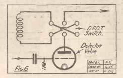
connect negative or positive L.T. to earth. The factor which determines which side shall go to earth is the valve. Some makers state that the "grid return should be positive because the valve functions best with a positive potential on
