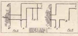
It is very simple. The aerial terminal of the set is connected via a fixed condenser to the loud-speaker extension circuit. That is all there is to it, but it should be noted that the choke and condensers are essential to this system.
