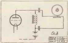
safety. A one-to-one ratio L.F. transformer can also be used, as shown in Fig. 4, but personally we prefer the choke-capacity method.
