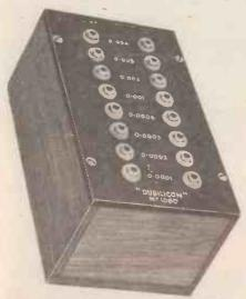
The Dubilier fixed condenser device known as the Dubilicon' which enables a large range of capacities to be obtained.
