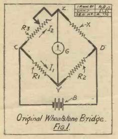
new footing. The new methods are, in fact, derived from the well-known principle of the Wheatstone resistance bridge, although the direct connection between the two does not at first sight appear obvious.
