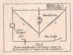
connected as shown, D being a sliding contact which can be made anywhere on the metre wire. The galvanometer will register a current for all positions of D,
