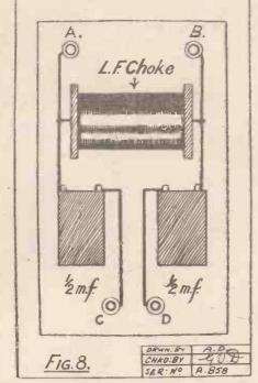
A and B should be connected to the 'phone or loud speaker terminals of the set, and the extension leads to C and D. The inclusion of such an instrument not only makes the wiring easier and safer, but actually improves reproduction, more
