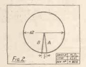
10<sup>3</sup>/<sub>4</sub> in., and cut this out with a sharp penknife. Take the paper cone and glue round the outside edge on the hollow side to a depth of about \( \frac{1}{4} \) in.; lay the cardboard ring flat on the table and fix the cone to this. At the same time press gently on the point of the cone to ensure getting it evenly spread out all round. When this is properly fixed give the whole a coat of spirit varnish, which will make it damp-proof and more solid all round.
