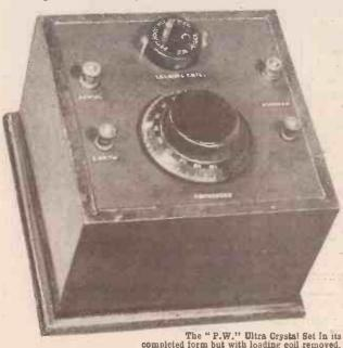
LIST OF COMPONENTS. d. 0 6 6 6 3 3 6 1 Panel,  $6 \times 6 \times \frac{1}{4}$  in. with box 1 Lamplugh '0005 variable con-17 denser Griphco '' permanent crystal 2 detector .. .. .. .. 2 Coil formers lb. 26 S.W.G. D.C.C. wire ... Bretwood single coil holder ... Screws, transfers, etc.
