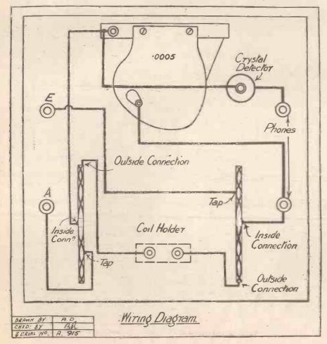
The 36 turns will leave a space of about in. on the outside of the former, so this should be trimmed off with a pair of scissors, except in the case of one section. This is left full length, a hole is made in the centre of it, and, when placed over the shank of the aerial or top 'phone terminal, and bent at right angles, this will hold the coil to the panel.
