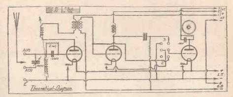
A similar group of impedances should be used if 2 volt or 4 volt valves are employed, and as separate H.T. plugs are provided for each valve and grid bias is included for the last two, each valve may be
