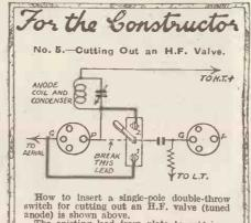
How to insert a single-pole double-throw switch for cutting out an H.F. valve (tuned anode) is shown above.
