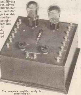
For this reason the first valve of this amplifier is coupled to the detector by means of an L.F. transformer, and the subsequent amplification is carried out by the resistance capacity method.
