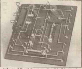
Another view of the back-of-panel connections which will be useful when wiring up.
