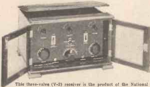
This three-valve (V-2) receiver is the product of the National Wireless Co., Ltd.
