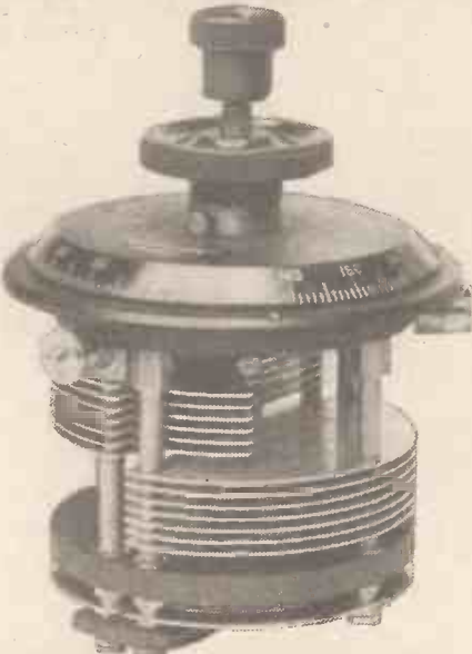
This double "Vanicon" condenser is eminently suited for the simultaneous tuning of H.F. circuits
