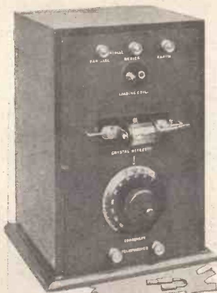
A photograph of the completed receiver. The shorting plug for the coil holder is seen in the foreground.
