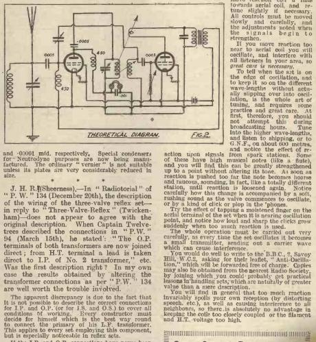
and 00001 mfd. respectively. Special condensers for Neutrodyne purposes are now being manu-factured. The ordinary "vernier" is not suitable unless its plates are very considerably reduced in size.
