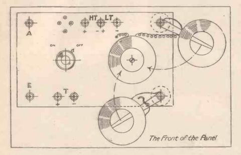
Coil No. 6 on the rod in front—they may all three be adjusted so that they lie exactly over each other with the Coil No. 6 on the top and Coil No. 7 at the bottom, adjustment of the two moving coils being taken up by means of two 2 B.A. nuts threaded on to the rods above and below the supporting strips.
