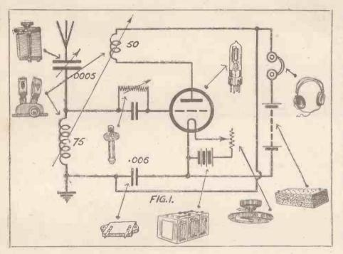
deviation from an ordinary detector circuit with reaction. Actually, if the 006 condenser be shorted and the lead from earth to reaction be removed, it does become a "straight" circuit, and for this reason is popular among amateurs, as this slight alteration allows them to get the circuit working well in its simple form before introducing the Flewelling element.
