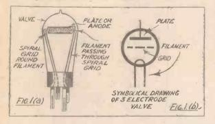
shows how a three-electrode valve is represented in electrician's diagrams.
