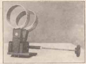
The two-coil holder with anti-capacity bandle.
