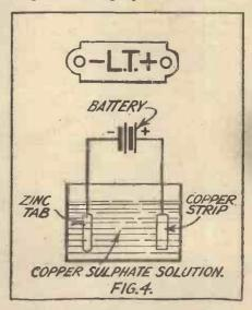
When the necessary writing has been carried out the varnish is allowed to dry heating will cause it to dry rapidly. The copper plating is then carried out exactly as before. When a sufficient amount of copper has been deposited, the zinc must be dried and then immersed in methylated spirit for a little while, so that the shellac becomes dissolved off the zinc,
