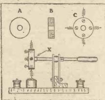
condensers, etc., which is drilled and tapped in the manner shown at B, and provided with four small clamping screws as shown at C.
