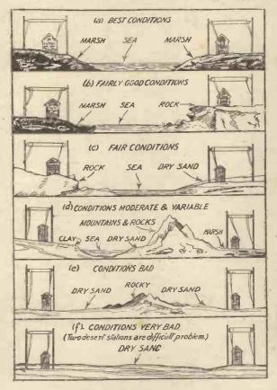
the other are the sandy, gravelly and rocky districts, where "earths" are difficult to arrange, and the reception is often poor, even when an efficient arrangement has been arrived at.
