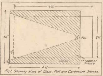
tin) foil,  $2\frac{1}{2}$  in. by  $4\frac{3}{4}$  in. Fix one sheet between two glass plates, using a little shellac varnish, allowing <sup>3</sup>/<sub>4</sub> in. of foil to project at one end (Fig. 1) Make four sets like this.
