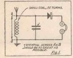
due to the fact than an auto-transformer is used so that the voltage across the detector circuit is made as high as practicable without cutting down the current flowing through the crystal, for it must not be forgotten that the crystal is a current operated device. This type of coil, which we have named the "Ultra" coil, is not only applicable to crystal sets, but also to valve receivers, and in various types and forms of circuits.
