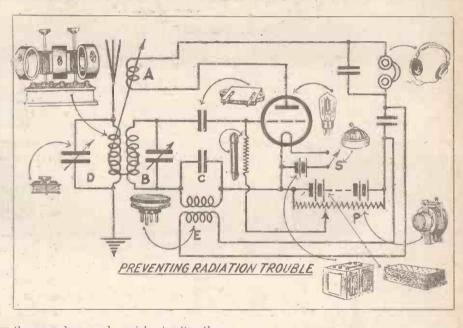
the secondary and aerial circuits, they cannot energise the aerial or be radiated from it in an undesired manner—i.e. so as to cause interference. The normal grid potential is initially adjusted by means of a tapping across the H.T. potentiometer shown, so that the change above described takes place practically instantaneously.
