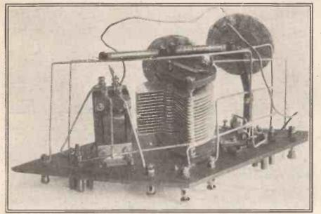
Fig. 9. The set completely wired up. Note position of fixed resistances.
