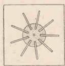
aside and forgotten; but with the aid of a little seccotine and a few wooden strips they can be made to serve as central hubs for "spider" formers of any desired size. The idea is clearly outlined
