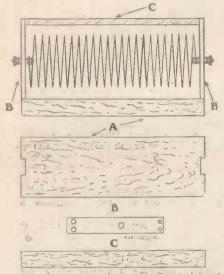
present-day tuning devices. Consisting of a formerless and open spaced coil of squaresection bare wire it is undoubtedly the ideal anti-capacity coil, especially for long distance reception; but, possessing a somewhat clumsy and none too plessing appearance, it is, for the present, confined to the experimenter's workshop, where it will, probably remain until its design is modified to suit the requirements of the greater majority.
