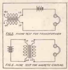
In the event of any wide differences being found, the transformer should be rejected or returned to the suppliers in exchange for another.
