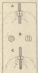
must be provided. The most usual method is indicated in diagram A where two lock nuts are tightened up on the rod and gripped in the vice. For the larger size rods this is usually quite satisfactory, but the threads of small rods are invariably stramed when the nuts are tightened up, and to avoid this it is best to split a nut by means of a hacksaw and use this as a clamp as shown at B and C.
