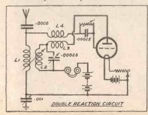
is stated that using dull-emitter valve and 221-volt H.T., local stations were received as loud as with an ordinary circuit using detector and one L.F., with reaction.
