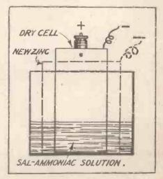
A dry cell treated in this-way will-often run for months; and when the zinc finally gives out, it can be replaced with a sheet of
