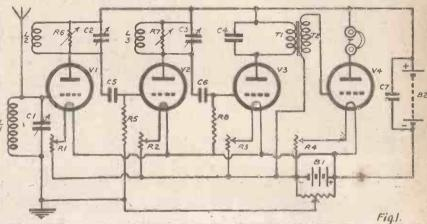
values of the variable condensers across the anode inductances, and by lowering the filament current or high-tension supply. It is also necessary to keep all the colls well apart, and also the leads which go to the colls. Figure 1 is the diagram of my receiver; the two tuned anode circuits are kept stable by means of the two resistances R.6 and R.7, which are variable. There are several types of variable resistances of 100,000 ohms which are useful for this. Figure 2
