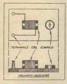
of the device, when the direction taken up by the needle will at once indicate the polarity. If desired, the solenoid may be made of fairly fine resistance wire, say any gauge between 30 and 40, or a resistance may be included in series with it, so that the current passing through the instrument shall not be large enough to cause damage to small dry batteries, for example.
