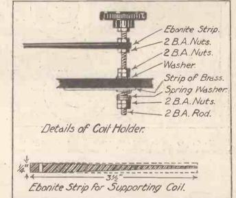
Two moving and one fixed coil are employed with holders as illustrated above.
