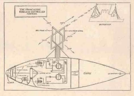
and therefore do not pick up any of these waves. On the other hand, No. 1 frame aerial is pointing north and south, and as the battleship is to the northward, one of the sides of No. 1 frame aerial is pointing directly at the battleship. Therefore this frame aerial will pick up a maximum amount of current from the battleship's transmitter.
