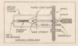
graphite coating is varied. The rubber strip is supported at one end by being tied to a bent brass strip frame, and the other end is secured to a wire stirrup which is attached to a cross-bar of fibre, ebonite, or glass. This cross-bar, which must be of insulating material, prevents the rubber strip from being twisted when the screw is turned. One terminal connects to the brass strip frame and the other to the wire stirrup.
