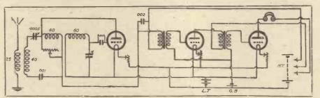
Theoretical Diagram of the 3-valve Filter Circuit.
