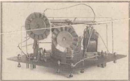
Fig. 8. The underside of the panel, showing completed coils.
