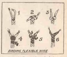
as shown in Fig. 4, the end of the tape being then slit longitudinally and used to bind up the separate leads as shown in Fig. 5. This makes a satisfactory and permanent job.
