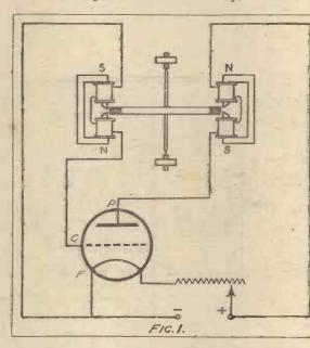
a motor of this type develops very little power, but apart from its interest, it can be used in experimental work, especially in physical laboratories where sometimes a wheel or disc has to be spun round with absolute freedom from sparking, which occurs even in the best of ordinary D.C. motors.
