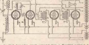
An ideal four-valve circuit, extracted from a Pamphlet published by Messrs, Ferrauti's, of L.F. transformer fame.
