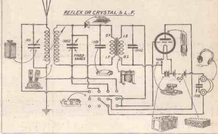
worked a loud speaker, but there was a certain amount of distortion with it, so I devised this circuit for loud-speaker work. I find that crystal and two-valve and one-valve amplifier. The switch-ing arrangement is fory simple-all switches up reflex, all switches down crystal and one-valve amplifier. Trusting this will interest you, I aun, yours faithfully, FREDK. W: WORTH. 41, Enu Road, Queen's Road.
