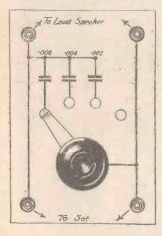
To suit the switching arrangement described later in the article it is necessary to choose capacities in the proportions of 1, 2, and 4; thus, 002, 004, and 008 mfd. would be suitable.
