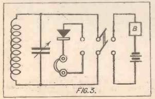
ser used in the instrument described is a Sterling "square law" type which has the advantage of greatly facilitating the plotting of wave-length charts.
