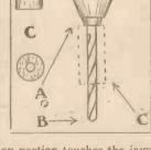
drill until the top portion touches the jaws of the chuck. It is thus impossible for the drill to cut deeper than the nieasured distance.
