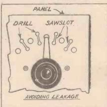
go right through the panel, and may be made quite large without seriously weakening the panel—they are cut when the panel is being drilled. In this way, accumulation of dirt or fine metallic particles, scraped off from the selector arm, which might cause leakage, is avoided. This little idea is taken from "Q S T," the journal of the American Radio Relay League.
