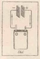
battery; this P.D. is equal to the E.M.F. of the battery, and in the case of the common type of "flashlamp" battery is about 4.5 volts. Before the plates are connected up there is no difference of potential whatever between them.
