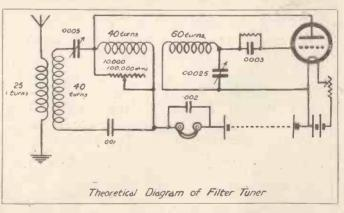
ohms less than one hundred thousand ohms will be O.K.; but as this instrument plays such an important part in the working of the receiver it should be thoroughly reliable, and no expense should be spared in its This resistance is utilised to purchase. control the strength of the magnetic field produced by the second filter coil, which, in turn, affects the entire filter circuit and controls, to a certain extent, regeneration and volume.
