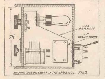
0003 mfd., in conjunction with a leak of 2 megohms, will always give good -results, if the filament and plate voltages are suitably adjusted.
