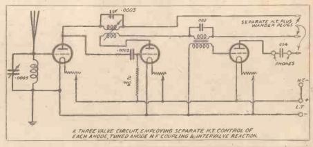
even to the anode of the second valve. Nevertheless, the second valve can stand a greater amount of anode potential, since the grid is already receiving a magnified
