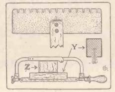
A slot cut with a single hacksaw blade is usually wide enough to accommodate the wire employed for winding frame aerials, but if, for other purposes, a wider slot is required then two or three blades should be fitted to the saw frame. which will usually accommodate three blades.
