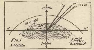
whereas he is forced, by practical considerations' of the size of his apparatus, if for no other reason, to make use of very short waves, in order to be able to concentrate them by the use of any system of conductors of reasonable proportions, the "Heaviside Layer," as it is called, being of unlimited extent, reflects all rays of whatever length.
