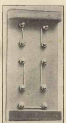
Showing the terminal connections under the panel.
