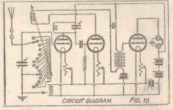
reception, and while tuning the set in it should be left with its knob about half-way round. When best results are obtained the potentiometer knob should be turned gradually to increase the signal strength.
