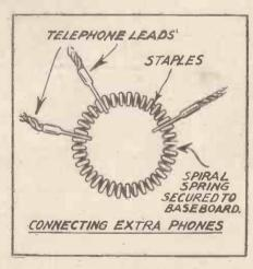
way. .The springs themselves may be made by winding fairly stout brass wire around any suitable cylindrical object, of a diameter of one-quarter to one-half of an inch.
