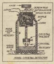
using a small bottle for the container, there is no danger of the mercury being upset or lost, and if any shaking occurs, as it is bound to do, the mercury automatically runs back into its proper place again. Only a very small 'quantity of mercury is required—a globule about the size of a shilling. A wire lead will be needed to pass alongside the cork, to make contact with the mercury. The crystal should be secured in the
