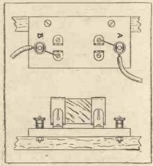
pairs of clips to take the interchangeable type of condenser. Two terminals, A and B, are connected to the clips as shown, one being joined to the aerial lead-in and the other to the aerial terminal on the receiver.
