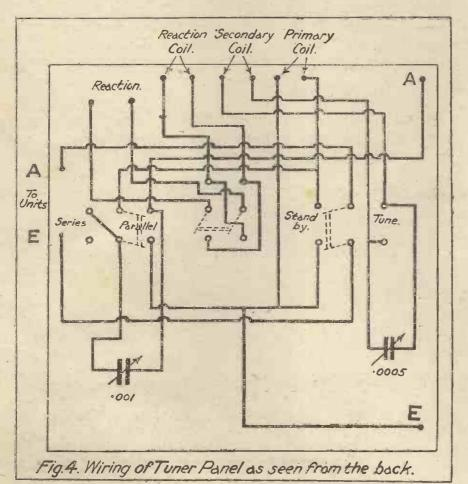
appear, where the tuner panel is viewed from the back. The switch positions are marked in this illustration, and it will be found convenient to mark the front of the panel correspondingly, remembering that the switch positions will appear reversed when
