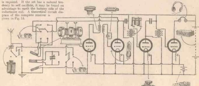
Fig. 15. Theoretical diagram of the Four-valve "Expanding" Set.-
