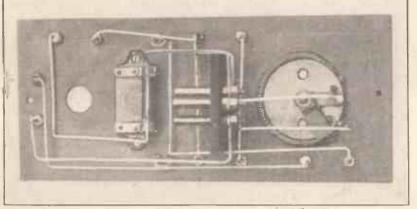
Fig. 9. Back view of detector unit. Reaction terminals are shorted if reaction not required
