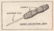
permit of their being slipped into position on the rod, as shown. The corks make a very good handle, and the tip of the rod should be filed to a suitable shape for the work for which it is intended.
