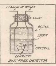
sent to me by a reader. It does two things, it keeps dust from gaining access to the crystal, and it also keeps the crystal free from grease, since the crystal is permanently
