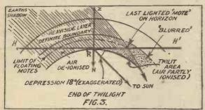
It will be seen at once that this time is considerably after sunset at the observer's position on the surface. Of course, the fading light and consequent de-ionisation does operate (in the lower layers) immediately after sunset to begin to improve reception. But it is not till the shadow reaches the Heaviside Layer that we are free from the effects of direct sunlight. We may call this time "Wireless Sunset" (see Fig. 4).
