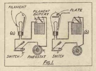
the velocity of their motion increases with increase of temperature, as also do their mean free paths. If the temperature of conductor reaches a certain value the surface tension is overcome and electrons leave the conductor. This effect may be compared to evaporation and we may regard the electrons as *boiled* out of the conductor.
