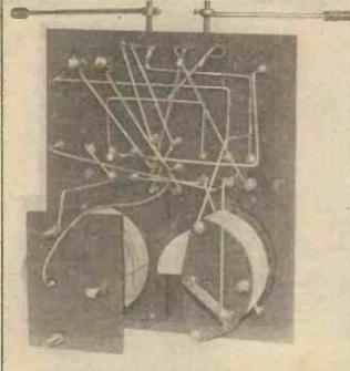
Fig. 5. The back of the tuner, showing wiring completed.
