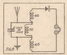
The following is a list of approximate values for various wave-length ranges, both the windings being tuned, the aerial with either series or parallel condensers of .0005. and the secondary with a 0003 or 0005 parallel condensers :
