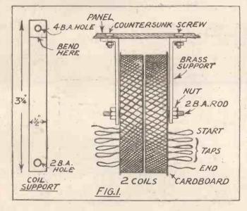
other is the secondary or crystal coil. The aerial is only roughly tuned, while the crystal circuit is tuned very finely by means of a variable condenser as well as tappings.
