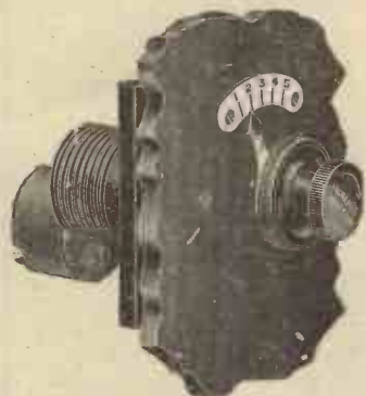
Combined Variable Intervalve reaction and Anode reactance. Wavelength range 200-4,000 metres. Price 45/-
