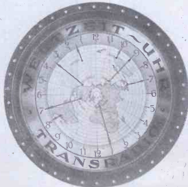
This wonderful clock is of German manufacture. The map is lit from behind, and a moving shadow indicates that part of the world where it is night. An arrow is drawn from each station's position on the map. Thus it is possible to gauge the time and whether light or darkness reigns at any of the large wireless stations in the world at a glance.
