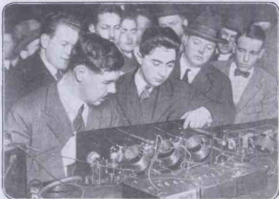
Prof. Hazeltine (left) examining one of his neodyne receivers. Enormous ranges without re-radiation are claimed for this wonderful instrument.
