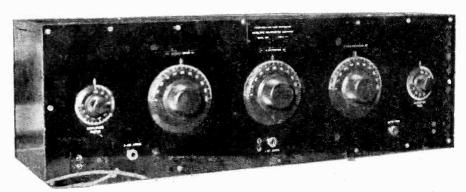
The external appearance of the Neutrodyne Receiver. The dial on the extreme left controls all the amplifying valves, no potentiometer being used, while the next dial controls the aerial tuning adjustment. The third and fourth are "neutrostages," and the last the detector valve control.
