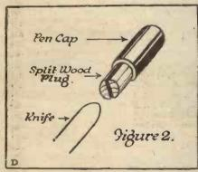
plug of wood longitudinally and push in the knife of the switch between the two halves of the plug. Fig. 2 shows the way this is done, quite clearly. If necessary, shellac or
