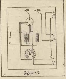
The panel is now ready for wiring. The wire used should be about 22 or 24 S.W.G. copper wire, and if covered with coloured systoflex will present a very neat appearance, and the insulation be the best. The low tension side should be wired first.
