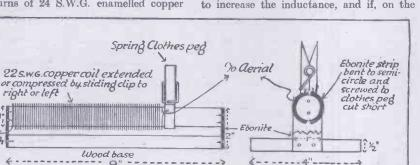
wire are wound on the ruler and then slightly slackened so as to fit easily, but not too loosely. One end of this coil is fastened to the ebonite support and then connected with the aerial terminal, whilst the other end is fixed to the sliding clip and then taken to the earth terminal. Meanwhile, the slider inductance coil is disconnected.
