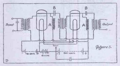
them down. It is best and cheapest in the long run to install a plate battery of small accumulators, or failing that, current from the mains or from a motor generator may be used, a system of choke coils and condensers being used to get rid of the hum. The owner of an ordinary note magnifier can easily convert this to a power amplifier,
