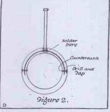
open them sightly to get the phones in between. This ensures a pincer-like grip of sufficient power to hold the phones securely in position.
