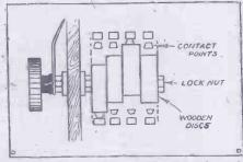
Before fixing the control knob to the end of the shaft, a pointer might be fastened between the knob and the washer and lock nut on the outside of the panel if it is desired. The contact strips are then fastened to a base in such a position that the turning of the knob moves the cam until it presses the contact strip against the second strip which is necessary to make a good connection to complete the circuit.
