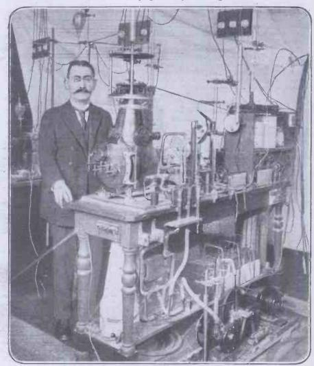
M. Dufour's invention, the cathode oscillograph, which is capable of recording the minute currents of highfrequency electricity.
