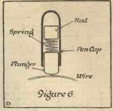
the wire on the inductance; the plunger is kept pressed on to the wire by a strong spring, which makes contact with the plunger and the rod going through the slider. Not fixed dimensions are given, these being determined by the amateur to the suit his own apparatus or fancy. This remark also applies to the other apparatus here described.
