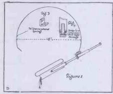
in more than uncomfortable and ill-fitting phones. To fit snugly but firmly to the cars each phone must have some sort of "universal motion" This is simply and effectively provided by what is known as the "stirrup and gymbal."
