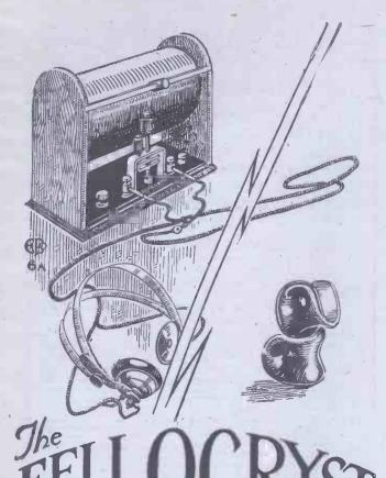
This is an excellent crystal receiving set, which gives very good results on all wave lengths from 300 to 1,500 metres, and is suitable for receiving broadcasting from ships and long distance stations.
