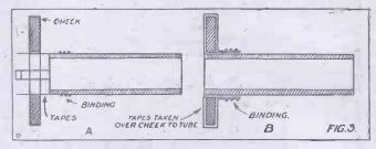
When this is done the core may be inserted in the bobbin, the first binding wire should not be removed to prevent the wires fanning out, but all the others should be removed as the core is inserted. When the core has been pushed through the bobbin, the first binding wire may be removed and the core adjusted to project equally either side.
