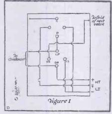
Fig. 1 shows the wiring of a typical high-frequency panel, the sockets at the top of the panel being for the valve and the lower ones for plug-in transformers. From this it will be seen that the plate of the valve is connected to one side of the primary of the transformer, the other side being connected to + high tension; across these two is a variable condenser.
