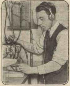
Detecting the presence of dirt by using wireless valves and telephones
