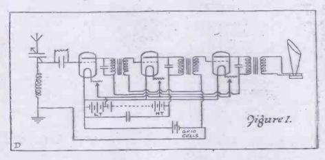
plished by means of a power amplifier, which is generally an audio frequency magnifier of special design, the name "power" being given to it because it handles currents which are comparatively large when compared with the currents thowing through the circuits of an ordinary radio receiver.
