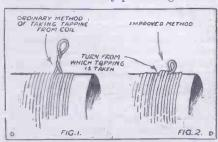
winding of the coil, bend the tapping down flush with the former and wind the follows ing two or three turns over the base of it. Then raise the loop of the tapping up again and continue winding the coil until it is desired to make a further tap, and so on, until the coil is completed.
