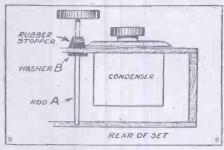
a way that it lays close to the rear of the front panel of the set as shown above.
