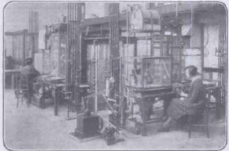
Testing Valves in the G.E.C. Laboratories, Wembley. The valve under test has a pressure of 5.000 volts D.C. on the plata
