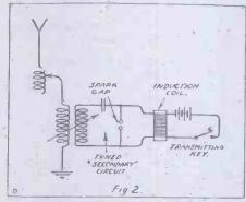
apparently simple device of feeding the spark discharges from a Hertzian oscillator directly into a long upright or "elevated" aerial. Such an arrangement will radiate waves which, when measured in metres, are equal to four and a half times the length of the aerial in metres. He used a similar elevated aerial to "pick up" the waves at the receiving end.
