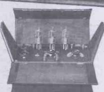
Highly efficient 3-Valve Broadcasting Receiver. Will tune in all the broadcasting stations and the low-wave French telephony.
