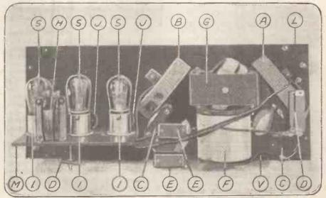
Fig. 1.—The various items that are required in the assembling of this Armstrong-circuit set are illustrated in this diagram. Note that the coil F and the variometer G are placed in inductive illustrated in this diagram. Note that the coil F and the variometer G are placed in induct relation to each other. The regeneration in the first valve is controlled by the variometer.
