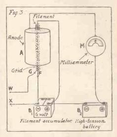
possible to explain here all the reasons why the three-electrode valve may be used as a detector or amplifier; it is only proposed to give a very brief theoretical description. It is found that if a positive potential is applied to the grid of a three-electrode valve, the electron current from the filament to the anode and round the anode circuit is increased, whereas if a negative potential is given to the grid the normal steady current round the anode circuit is decreased.
