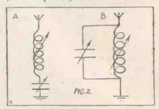
is used as a rough tuning device, and the variable condenser as a fine adjustment.
