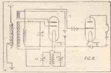
Fig. 6 .- How super-regeneration may be obtained by varying both the damping and the regeneration with respect to each other, keep-ing the proper phase relations.
