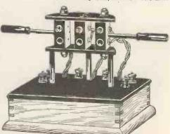
The illustration is that of our Three Coil Holder Complete Unit for use with any standard coils, mounted on malogany base, with ebonite top and well lacquered brass parts. The levers at the side make possible the most critical adjustment with the very minimum of friction.
