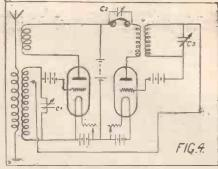
Fig. 4.—This diagram illustrates the method of obtaining super-regeneration by varying the damping of the first tube circuit with respect to regeneration. The set described in this article uses an adaptation of this method.
