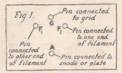
called a grid. This grid is a metal structure arranged between the filament and the anode, and is of open-work nature so that electrons can pass through the holes in the grid on their way to the anode.
