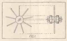
The next consideration is the number of spokes, which is determined by the size of wire with which the coil is to be wound. If thick wire is to be used on a small-sized coil nine spokes are sufficient, but this should be increased to eleven or thirteen for larger sizes employing finer wires. The chief point to remember is that the number of spokes must be odd, as otherwise the coil will not take up a basket formation; in fact, it will be impossible to wind it unless this rule is observed.
