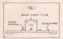
The receiving apparatus for use in connection with the wireless control of a model electric train will consist of a coherer, relay, simple selector (i.e., selection by sequence), and switch, the latter for opening and closing the circuit connected with a coherer. Current for the coherer circuit will be supplied from an ordinary 3½-volt pocket-lamp battery.
