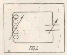
the non-conductor as the "dielectric." Such simple components being required, it follows that very numerous types of condensers can be made. The dielectric may be of mica, ebonite, glass, oil, or air, each of these materials having an arbitrary numerical value as a dielectric. This value is called the "dielectric constant" of the material, and the scale of values is arrived at by assuming the constant to be I in the case of air.
