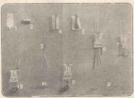
The various parts of the valve before assembling.
