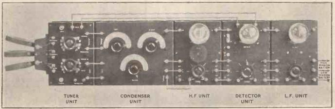
The Panel Unit System Receiver, manufactured by Messrs. Peto Scott.
