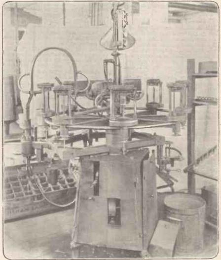
The sealing-in machine, in which the "pinch " is sealed in a valve. (See special article on page 475.)
