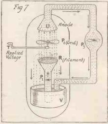
main propeller H revolving at the same speed. The distance between U and R weakens the suction effect on water emerging from the rose R; but the propeller P<sub>2</sub>, being quite close to R, has a very big effect on the quantity of water sucked up into the funnel U.
