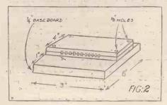
you have two slotted sections exactly the same size. Place the slotted sides face to face squarely, and stand them upon the other sheet of ebonite (6 by 3 by \frac{1}{4} in.) which forms the baseboard. If they are placed in the centre there should be an inch clearance at each end of the latter, and the whole
