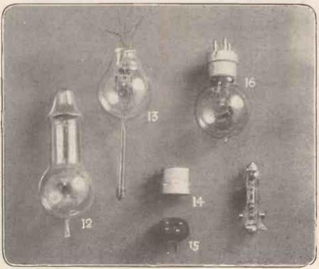
The valve nearing completion: The last phases in its construction,
