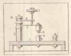
The parts F and K are two crystal cups. These can be bought of any wireless dealer, or can easily be made from old brass cartridge cases.
