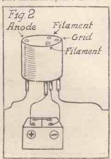
plate; the two pins marked F<sub>1</sub> and F<sub>2</sub> are connected to the two ends of the filament wire. Sometimes the valve will have the cap lettered showing which pin goes to which electrode; sometimes the pin going to the anode is indicated by the letter A or P. The pin immediately opposite is the grid, while the other two are the filament pins.
