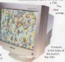
Sony MultiScan 400PST. Attractive, and with a full 18in viewable diagonal Trinitron tube, this monitor has both D-SUB and BNC connectors for connecting it to two computers at a time, and there is little variation in picture sharpness across the screen. A comprehensive and easy-to-use on-screen display with a 75Hz non-interlaced refresh rate at 1600 x 1200 resolution, makes this monitor a joy to use.
