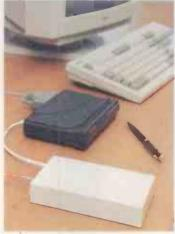
■ Telefficiency claims its eSaver helps internet users cut phone bills by routing calls via the cheapest network. The device fits the modem and the phone socket. Telefficiency offers local call rates at a claimed 20 percent cheaper than BT's. Its ePlan 18, which includes the service and the device, is £18 per year.
