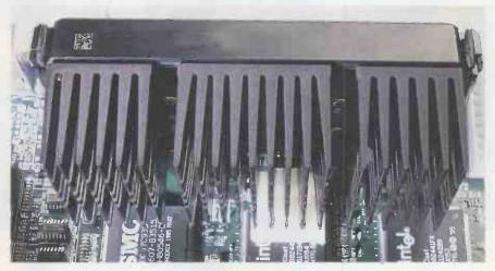
The Pentium II processor is big and fast. Note the size of the heatsink and the way the cartridge, encasing the processor, sits upright
