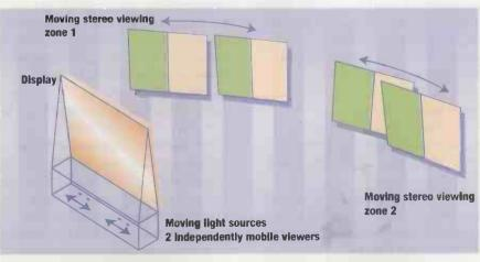
Fig 2 A diagram of a display designed for two people, the green half of each panel representing what would be seen by the left eye of each viewer, the red half by the right eye. A tracking device would independently monitor the movement of each person viewing the Image, and move each of the two light sources correspondingly
