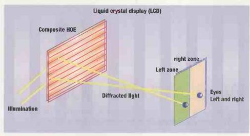
Fig 1 A simplified diagram of how the display works
