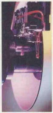
Inside an OAW drive — note the optical fibre. MO drives normally use an open beam
