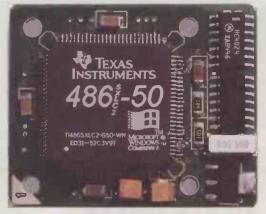
Technomatic is selling a kit claiming to upgrade 386 and 386SX machines to 486 performance for just £99. The kits, from Workstation Source, comprise a Texas Instruments SXL2-50MHz chip sitting on a tiny daughterboard. This replaces a 386DX chip or "piggy-backs" a 386SX up to 25MHz.
