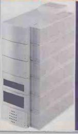
The modular expansion chassis is designed so that capacity can be increased by stacking additional interlocking disk modules. Each disk module is removable for hot swap and portability. The system can operate with a single module and expand to keep pace with growing system demands. As many as seven modules can be stacked in a SCSI chain. The system provides for up to 45GB of fault tolerant storage. Support is provided for: Netware NT WINDOWS SUN SG APPLE IBM...
