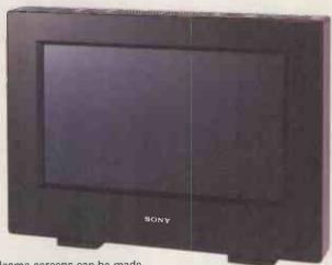
Plasma screens can be made very thin, and Fujitsu has even developed a 50in plasma panel. But plasma displays can cost ten times more than a CRT device and tend to be used in specialist areas such as aeronautics.
