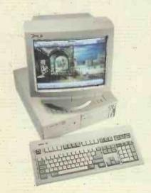
ewlett Packard is a company better known for its expertise in the printer market than for building PCs. Vectra is the name of a series of multimedia PCs produced by HP, all of which come with an integrated speaker, SCSI CD-ROM drive and an audio front panel with jacks for headphones and microphone.
