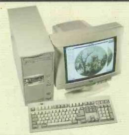
A the front of this machine, believe it or not, there's a graphic equaliser, or more specifically, the Equaliser Amplifier Pro from Platinum. It has seven bands, a volume and balance control, and aims to turn your PC into the full-range, stereo, 60W sound machine that multimedia PCs always promised to be.
