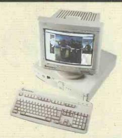
his is the desktop version of Mesh's DX2/66 multimedia machine. Inside, everything is fairly standard with the lefthand side of the box housing the motherboard, processor, and card slots while the righthand side holds the power unit and Sanyo CD-ROM drive. In the centre sits the disk drive with a 730Mb Western Digital hard disk underneath.
