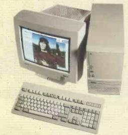
he first thing you notice about this machine is its built-in security features. On the front there's a lockable door which prevents access to the CD-ROM and disk drive. To the left of the drives there's a large power switch and below it are the usual reset and turbo buttons, but there's an extra button which allows you to disable the keyboard before locking the door. These features can be handy, but of course, they won't stop anyone from running
