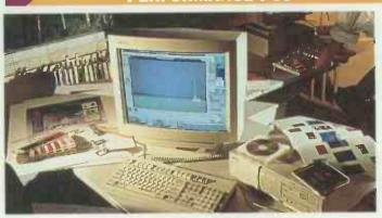
The new HP Vectra VE offers Intel Pentium 75MHz CPUs with PCI bus interconnection for the graphics and hard disk subsystems. To further increase performance, a secondary cache of 256 KB and video DRAM memory may be fitted. All HP Vectra VE Pentium PCs come with 8MB RAM as standard and MS DOS 6.2 with MS Windows for WorkGroups 3.1 pre-loaded.
