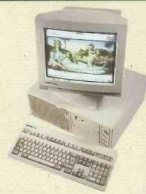
eacock and AST are the only two manufacturers in this group test to submit machines using Cyrix processors. This machine's CPU, though, stands out in another way - it's a DX2/V80. According to Cyrix, it offers up to 35 percent. improvement over an Intel-based DX2/66 for the same price, which is why we decided to include it here
