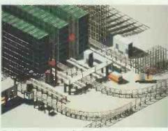
This Lego-like model of an industrial process was produced by the Taylor II simulation package, which won a Best of Cebit 95 award. Dutch developer F&H Simulations (+31 1336 6344) says a big selling point is its capacity for dynamic analysis of complex processes
