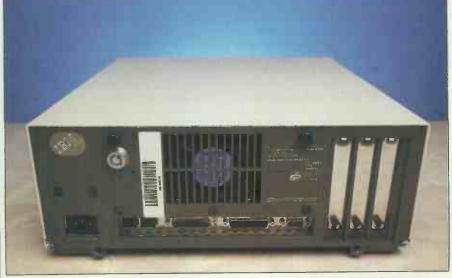
All the standard ports run off the motherboard, freeing slots for further expansion. From left to right: keyboard, mouse, bi-directional Centronics, RS232C and video out. The centrally-mounted fan is almost noiseless
