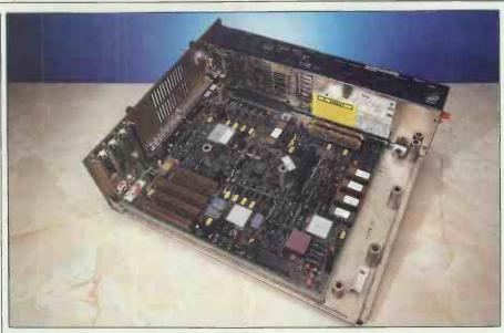
Surface-mount technology features large inside the Model 50, making the machine cheap to manufacture and expensive though not impossible to clone. Subsystems within the box are easily installed and removed
