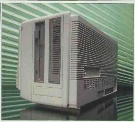
One of the major reasons for the Compaq's 'larger-than-lapheld' design is the inclusion of a standard 51/4in disk drive
