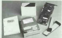
A 20 megabyte hard disk drive has the storage Gapacity of 50 floppy disks and is 10-12 times faster than a floppy disk drive. it enables you to store a whole programme/data library inside your micro. Floppy disks need only be used for back-up storage. In essence, a hard disk drive can transform the way you work with your micro.
