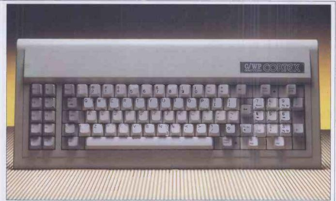
Keyboard is a direct IBM imitation; note the LED in the caps lock key.
