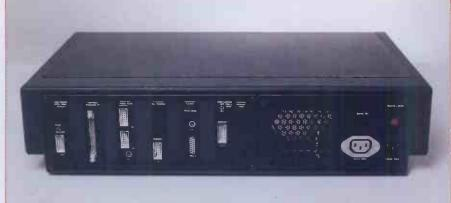
Peripherals plug directly into the circuit boards which form part of the back panel.
