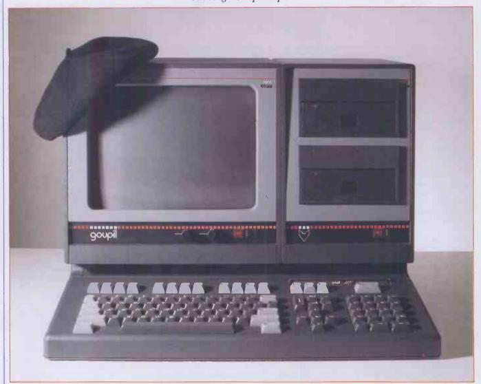
The Goupil-3 is a modular computer system designed to cater for both professional and personal needs. Its building block design allows the user to build up a computer system from the simple screen, console and keyboard configuration to a fully expanded system supporting three processors, a choice of six operating systems and offering multi-user and multitasking facilities.
