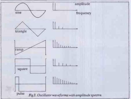
the required waveform. There is no fundamental limitation to the complexity of sounds that a digital synthesiser may produce.
