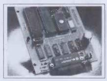
FOR EPSON PRINTERS, Microbuffer/E inside the existing auxiliary slot comes in two serial versions 8K or 16K (upgradable to 32K) and two parallel versions - 16K or 32K (upgradable to 64K). The serial buffer supports both hardware handshaking and XON-XOFF software handshaking at baud rates up to 19,200. Both interfaces are compatible with standard Epson commands, including GRAFTRAX-80 and GRAFTRAX-80 + . Prices range from \$159 to \$279.
