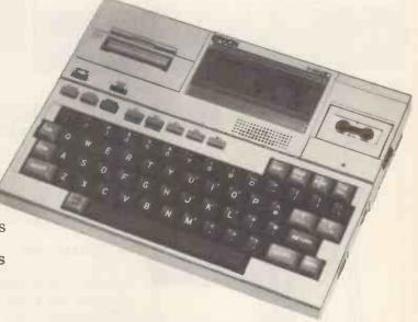
A computer small enough to fit into a briefcase yet with a full size typewriter keyboard, LCD virtual screen, printer and microcassette facility actually built in. High speed serial communication with other computers plus the Epson reliability – a world beater.
