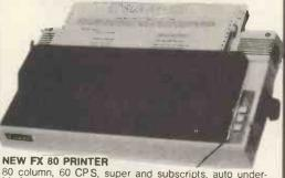
80 column, 60 CPS, super and subscripts, auto under-lining, tractor feed, 32 print fonts. Bi-directional printing, logic seeking, 9 x 9 matrix, high res. graphics, centronic parallel interface, tractor or friction paper feed. FREE 500 sheets of paper ... Price: £379 + VAT = £435.85
