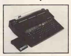
The T/Printer 35 is the lightest weight and lowest cost daisy wheel printer you can buy for your computer. So it will fit within your budget and you can carry it wherever you take your micro. Yet it is tough enough to give years of reliable service. Interchangeable typefaces (standard Olivetti 100 character daisy wheels), variable pitch, multiple copies—all the features you would expect of more expensive word processing printers.
