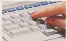
A typewriter-style keyboard incorporates characters and symbols plus a numeric key-pad and ten user-definable keys for fast and simple operation.
