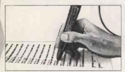
Bar code reader. A quick and easy way of loading any one of the software packages. The wand simply lifts' the coded program straight off the page of your HP-41C solution books.
