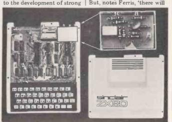
Welsh Sinclair addicts Gwynedd Computer Services have 'designed and implemented', so they claim, 'the definitive solution to the perennial Sinclair ZX80 cassette interfacing problem.' This pic shows where their little circuit fits into the white box, costing £9; and there is an installation and testing service which costs an extra £3. Details on (0248) 810748.
