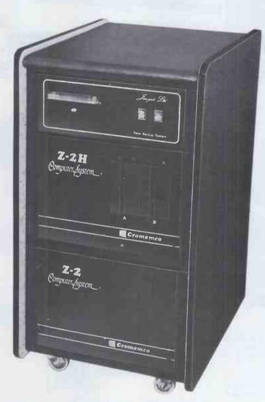
With the Jarogate Z2-HMP, each user has his own full CPU with 64k/bytes of RAM (CP/NET plus 60k of available user memory). And there's a high-speed parallel bus giving fast interprocessor communication so that users can have access to the central disk resources without the usual communication bottlenecks.
