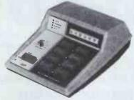
This unit provides simple, reliable programming of up to 8 EPROMS simultaneously it has been designed for ease of operator use — a single 'program' key starts the self check — blank check —
