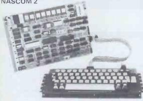
Kit includes all parts to build CPU board which has resident 8K Microsoft BASIC and 2K NAS-SYS 1 monitor for machine code programming. Included with kit is a fully assembled LICON QWERTY SOLID STATE KEYBOARD specially designed to exploit the potential of the NAS-SYS monitor. Other interfaces include video to monitor or domestic TV, Kansas City standard cassette interface (300/1200 baud) or R\$232/20mA teletype interface and two uncommitted parallel ports.
