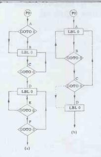
Fig 1. Multiple use of GOTO/LBL combinations. In Fig 1(a) execution will follow routes A-B, C-B, E-D and F-D. In Fig 1(b) the route C-D is invalid. NB, for convenience, the logical jump tests are not shown.
