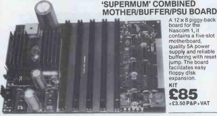
A 12 x 8 piggy-back board for the Nascom 1, it contains a five-slot motherboard, quality 5A power supply and reliable buffering with reset jump. The board facilitates easy floppy disk expansion.
