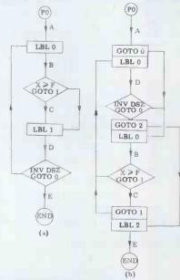
Fig 3. Reverse sequence programming.
