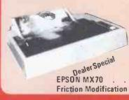
\*5x7 dot matrix \*80 CPS uni-directional \*96 chr set inc £ sign \*High Resolution Graphics (8x480 dots/line) \*80 chrs/line or extended \*Adjustable Tractor Feed \*4" to 10" paper with up to 3 copies \*Easy head replacement. Ideal for Acorn, Apple, Nascometc.
