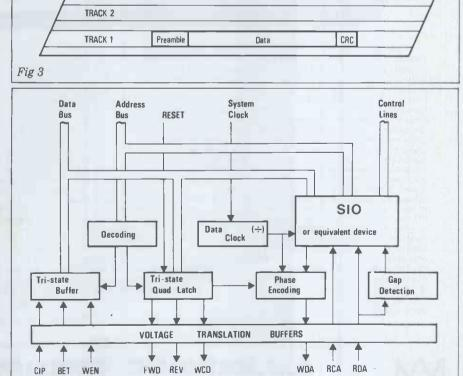
used in most disk systems. The file is then written into the first available free blocks on the tape. After each block is written the tape is backspaced and the block is read and the CRC checked, giving automatic verification.
