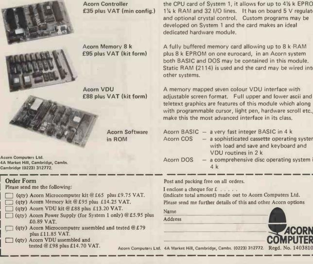
the CPU card of System 1, it allows for up to 41/2 k EPROM, 1¼ k RAM and 32 I/O lines. It has on board 5 V regulator and optional crystal control. Custom programs may be developed on System 1 and the card makes an ideal dedicated hardware module.
