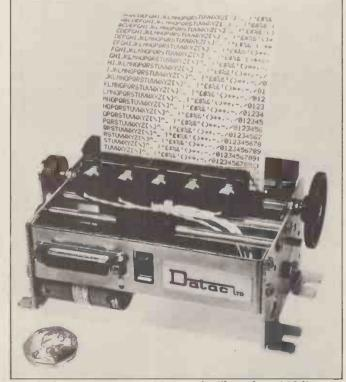
This little print unit costs £139, and will produce 120 lines of output a minute with its five print heads. It needs drive circuitry, and it is available without this from Datac on 061 941 2361.
