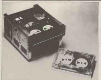
Attempting to catch up with the outside innovators at Courtest, the 3M Company has announced a disc-like tape cartridge as "the first truly intelligent data cartridge drive system". It differs from Courtest's in offering 16 track recording, and in being rather slower; also in being offered purely as a back-up system for the new mini hard discs, rather than as a systems component functioning in real time. There are other differences too. Details on 0344 58550
