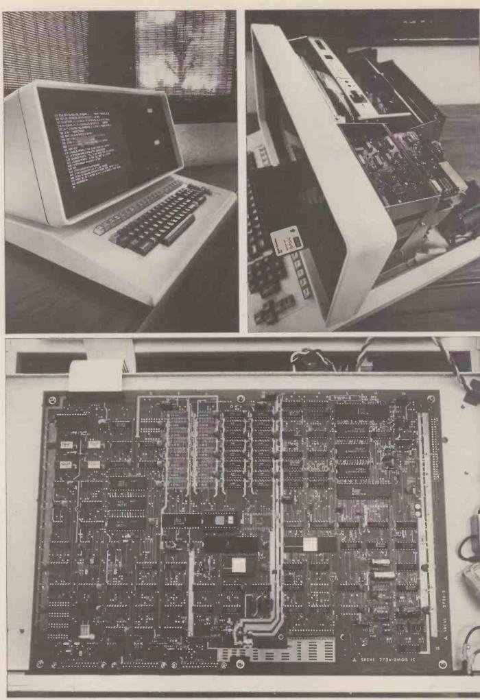
Top left: a general view of the Panasonic JD-700U; note the top row of user-assignable function keys. Top right: a peep inside shows the usual arrangement of disc drive, PSU and CRT. Bottom: revealed, the single board computer, with 8085A, 2MHz CPU, memory and all the circuitry for the disc drives, CRT and three RS232C ports.
