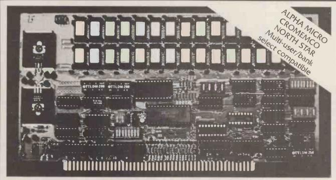
Model DMB-6400 Series dynamic 64k byte RAMS incorporate the features which are standard in the DM-6400 Series and adds bank select for multi-user-timesharing applications.
