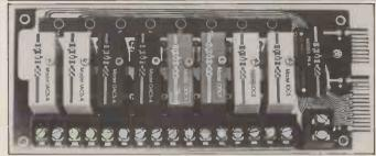
The five volt power supplies of micros need protection from the higher voltages used for industrial control: this input-output module from Rapid Recall will do that. Outputs up to 3 amps at up to 140V, inputs up to 130 V are converted to micro levels.
