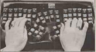
Arrange the standard typewriter's keys like this and it goes 40% faster—fast enough to type at dictation speeds. On this theory, the Department of Trade and Industry has bought ten word processors using the keyboard from PCD in Farnborough, at £7,000 each. If this pre-production test goes well, PCD hopes to push this "Trolley Dictation Concept" into the normal word processing market as well. Details on 0252 511001.
