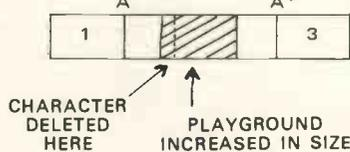
The character is deleted at point A. The playground is increased in size by one character and point A moves one character further away from point A<sup>1</sup>. Note that insertion and deletion are compensatory in their effects on playground size.
