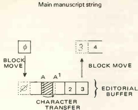
To move backwards, block 3 is transferred back to the main string and block 0 is transferred to the editorial buffer. Character transfers occur as in Fig. 3B to move the playground to the point of interest.
