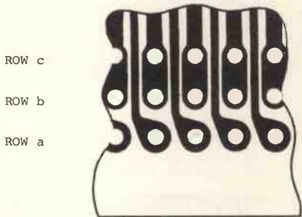
Fig. 2 Pad Configuration to Accept 64/64 and 64/96 Connectors
