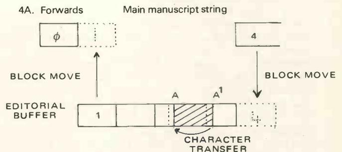
To move forwards, block 1 is transferred back to the main string and block 4 is transferred to the editorial buffer. Character transfers occur as in Fig. 3A to move the playground to the point of interest.
