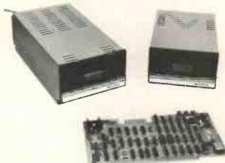
Micropolis disk drives employ higher standards of engineering to pack either 143K or 315K bytes per diskette, formatted. Supplied complete with controller card, cables, manual and software they plug directly into the S100 bus; 8080 or Z80.
