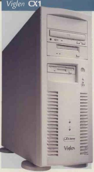
PRIOR TO THE RELEASE of the CX-1 in 1999, Viglen had always insisted on using Intel motherboards in its servers, but this time around it has opted for a SuperMicro board. The P6DBU
