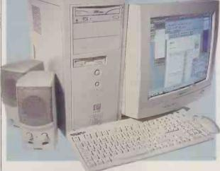
EVESHAM.COM'S entry this month is built around the popular 700MHz Athlon processor, mounted on an MSI K7 Pro motherboard. The MSI board is based on AMD's own 750 chipset and backed up by 128MB of PC100 SDRAM in the form of a single DIMM module, with two DIMM slots free. A Diamond 56i Pro modem and SoundBlaster 128 sound card occupy two of the PCI slots, leaving two. Access to these is unhindered, as evesham.com's engineers have neatly routed all cabling.
