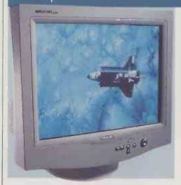
ON PULLING THE Philips 107P out of its box, the first thing that strikes you is the styling of the unit. With limited desk space in mind, the 107P is designed with a narrow back and sweeping flanks that curve to the front of the chassis. The bezel is also quite narrow making the screen look much bigger than it really is. On the front are some unusual silver OSD controls comprising four arrow keys and an 'OK' button. Even the flimsy on/off switch has had the silver paint
