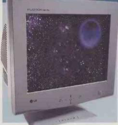
CONVENTIONAL CRTS are still based on a screen that is formed from part of a glass sphere – or a cylinder for Sony's Trintron displays. However, some screens are designed with a completely flat front surface such as Mitsubishi's Diamondtron NF and FD Trinitrons. Although these tubes can produce wonderful results, the internal surface remains curved to compensate for beam diffraction. This is where the LG Flatron differs as both sides of its tube are flat.
