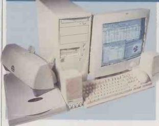
AT THE HEART of the Advent system from retailer PC World beats a Pentium III 650MHz mounted on a Gigabyte GA6 BX7 motherboard. The system also comes with a single 128MB PC100 SDRAM module residing in one of the three available DIMM slots.
