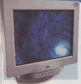
THE PR705F IS A 17in member of CTX's ProFlat series, all of which sport an 'absolutely flat screen'. Not only is it flat, but the fascia is constructed to highlight this, with sharp edges and barely a curved surface in sight. The only curves visible from the front are where the OSD control buttons are situated. At the back of the unit, along with the D-SUB input are BNC connectors for RGB input. The unit also conforms to the TCO99 standard.
