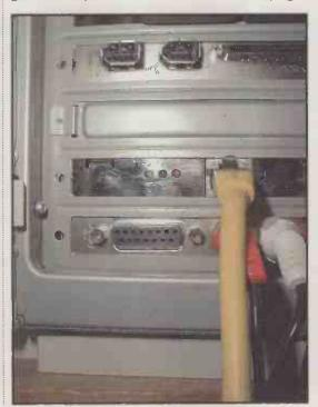
detects read or write activity on the network, even when there is no activity on the adaptor. If the ACT LED is not on, make sure that the hub and network are operating and that the correct drivers
