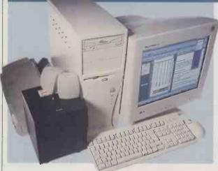
THE VISION EDUCATION A700 is the first machine we've seen from Multivision and, as the name suggests, its Athlon processor is running at 700MHz. The motherboard is a K7 Pro from MSI. The modem and the SoundBlaster PCI 128 fill two of the five available PCI slots on the board (with the sound being pumped out to Labtec speakers), which leaves three free PCI slots for upgrading. Memory comes in the form of a single 128MB PC133 memory module, fitted into one of the
