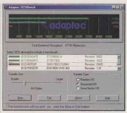
Adaptec's SCSI-bench shows the relative performance of sequential data transfers on three disks on my system – note the Ultra160 drive is sustaining more than double the throughput of my older U2W drive, while an ancient SCSI-2 drive has virtually given up the ghost
