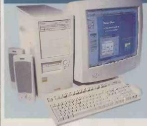
CARRERA HAS SUPPLIED a machine that boasts the largest monitor – a 19in LG CS990DC. With a tube that isn't flat in any direction, this shadow-mask unit doesn't stand up to some of the vibrant and sharper aperture-grille models on test here. It may also be on the bulky side, if your desk is small. However, if image manipulation is a priority in your studies, you'll like the extra screen space.
