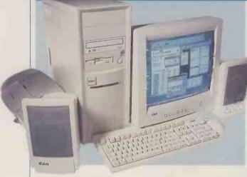
ABSENT FROM OUR group tests for seven issues, Dan Technology returns with a machine that features Intel's Flip Chip. This FC-PGA (Flip Chip Pin Grid Array) Pentium III is clocked at a respectable 700MHz, with 256KB of full-speed Level 2 cache squeezed on the die. With 128MB of PC100 memory leaving two DIMM slots free, the Dan is a mid-range performer sitting in the middle of the SYSmark 2000 results.
