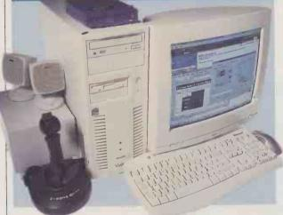
FITTED ONTO AN MSI MS6119 motherboard is the most powerful processor in this month's group test: an 800MHz Pentium III. Using this raw power, the Viglen sits comfortably at the number one spot in the SYSmark Internet content creation table. The Homepro's weakest area was 3D, where it slipped towards the bottom end of the tables. But even taking this into account, its overall performance can only be considered to be impressive.
