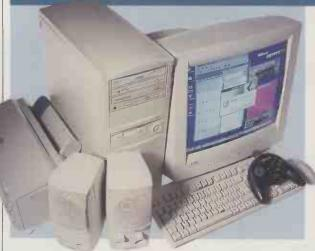
SIMPLY'S ENTRY easily topped both the Quake III and 3DMark tables. Bearing in mind that the system employs the same Creative 3D Blaster Annihilator Pro with 32MB of DDR memory as some of the other machines, the results cannot be ascribed purely to the graphics card. Although in combination with the Athlon 750MHz, the AOpen AK72 motherboard and the 128MB of PC133 SDRAM, the system performs extremely well. For the student with a gaming interest, Simply has also
