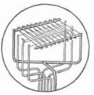
Typical Electrodes of Marconi Power Valve.
