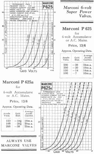
NOTE: Anode Volts-Anode Current Curves for P625 & P625a on p.43.
