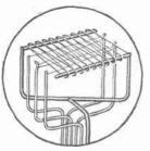
Typical Electrodes of Marconi Power Valve.
