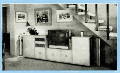
SOUND UNDER THE STAIRS — In this installation the speakers are mounted at each end and the adjustable doors reflect the sound into the room. The television chassis is rotatable, stereo radio, tape and record reproduction is provided (H. H. SCOTT).
