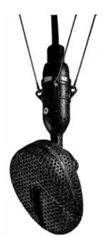
The 4105 microphone is a moving coil pressure-gradient microphone with a cardioid response obtained by using an acoustic phase shifting It is small. network. unobtrusive and robust.
