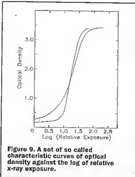
Figure 9. A set of so called characteristic curves of optical density against the log of relative x-ray exposure.
