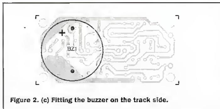
Figure 2. (c) Fitting the buzzer on the track side.
