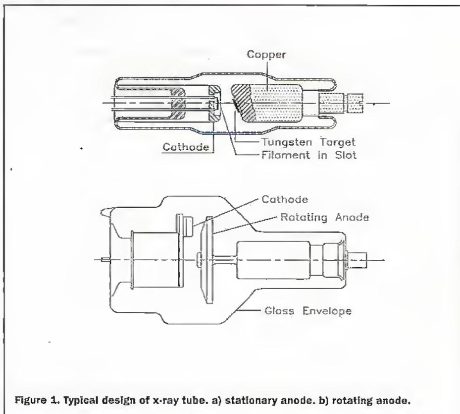
Figure 1. Typical design of x-ray tube. a) stationary anode. b) rotating anode.
