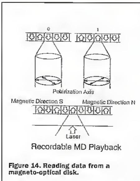
Figure 14. Reading data from a magneto-optical disk.
