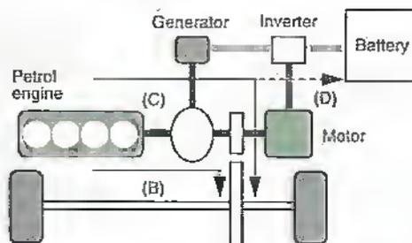
(D) If battery charge is low, engine power is used to generate electricity to charge battery.
