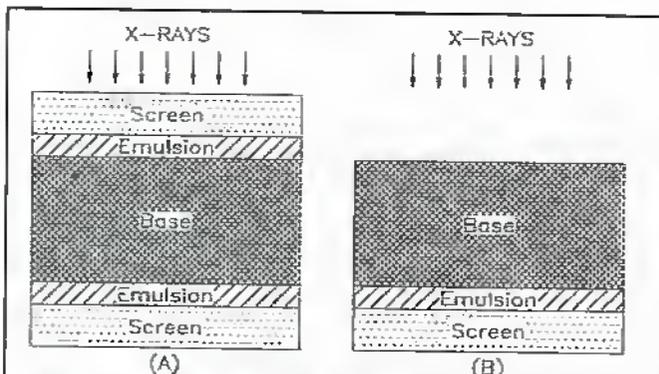
Figure 10. Utilisation of double (A) and x-ray single screens (B). The double screen provides for the highest sensitivity though the single screen provides for a sharper image.
