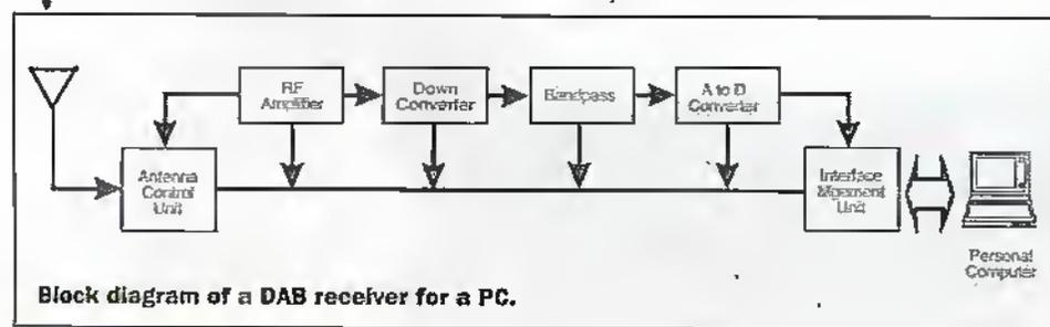
Block diagram of a DAB receiver for a PC.
