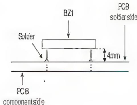
Figure 4. Mounting Buzzer BZ1.
