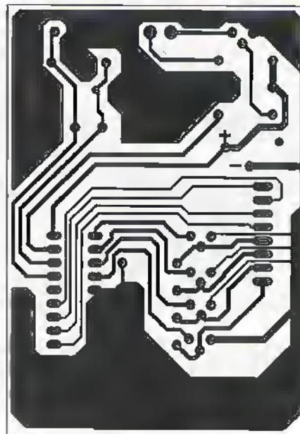
Figure 8. Underneath copper layer for transmitter PCB.
