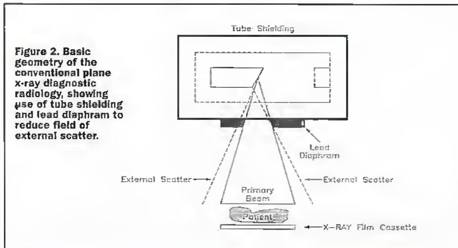
Figure 2. Basic geometry of the conventional plane x-ray diagnostic radiology, showing use of tube shielding and lead diaphragm to reduce field of external scatter.
