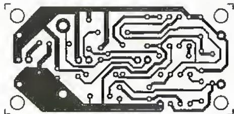
Figure 2. PCB Layout (a) Track.
