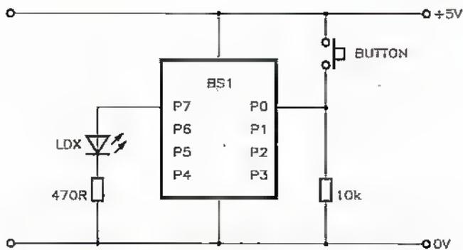
Figure 4. Using input and output to build a simple control application.
