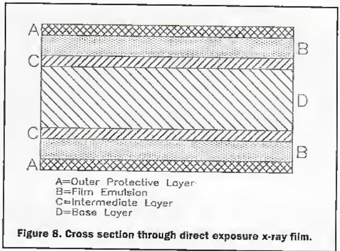
Figure 8. Cross section through direct exposure x-ray film.
