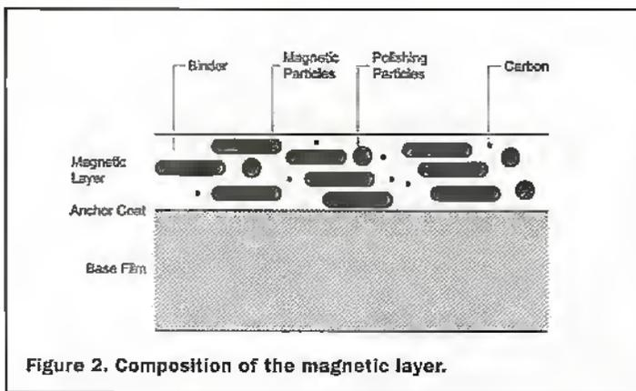
Figure 2. Composition of the magnetic layer.
