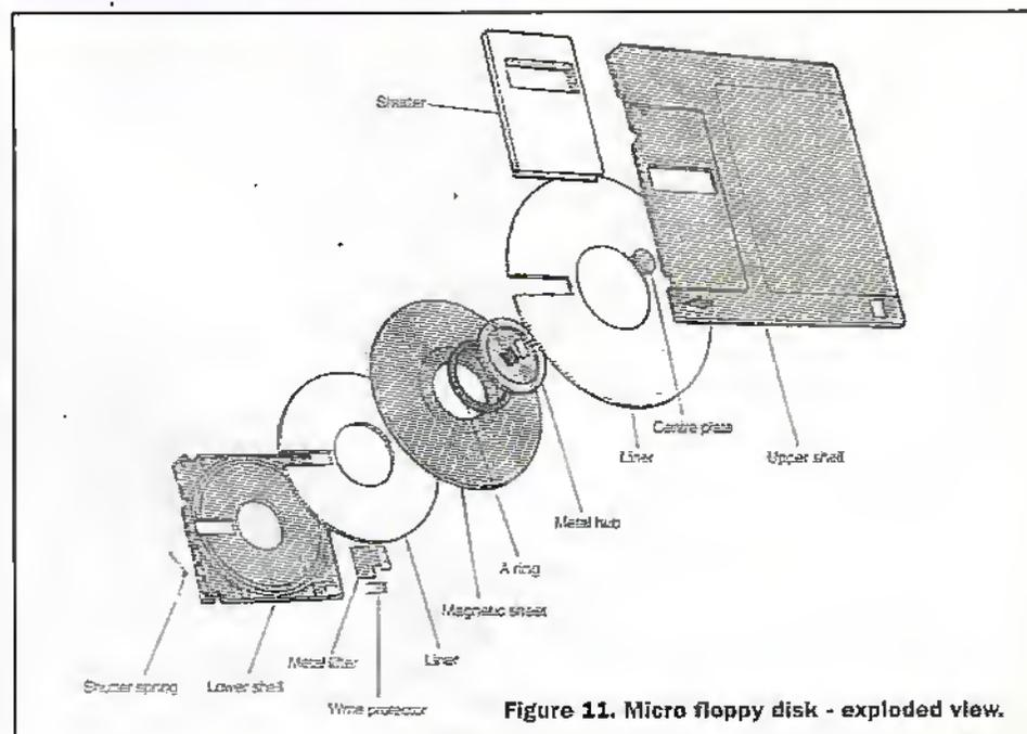
Figure 11. Micro floppy disk - exploded view.
