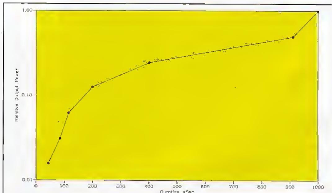
Figure 1. Power Output Vs Duration of Flash.
