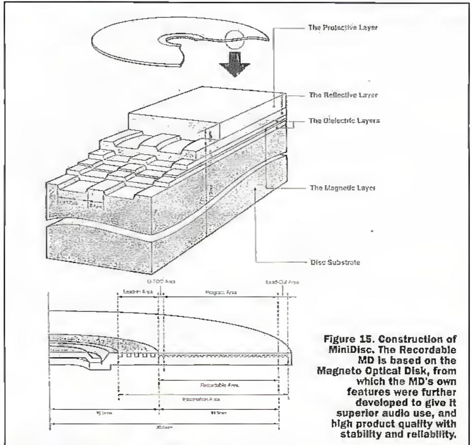
Figure 15. Construction of MiniDisc. The Recordable MD is based on the Magneto Optical Disk, from which the MD's own features were further developed to give it superior audio use, and high product quality with stability and reliability.
