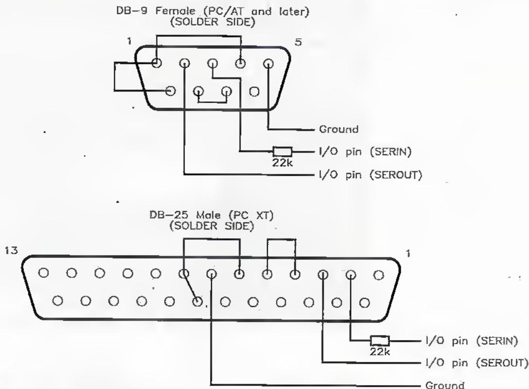
Figure 7. 9 and 25-pin serial connection to a PC.
