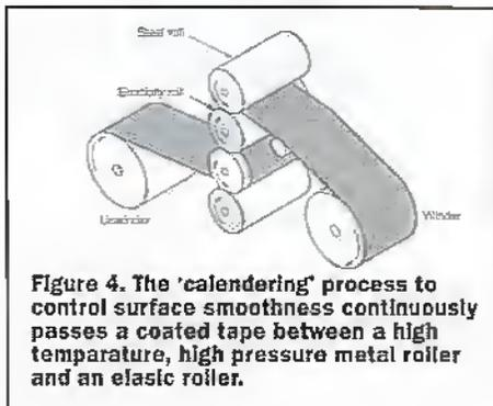
Figure 4. The 'calendering' process to control surface smoothness continuously passes a coated tape between a high temperature, high pressure metal roller and an elastic roller.
