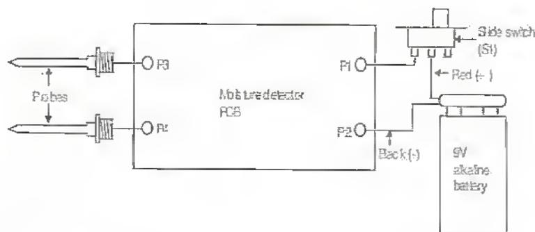
Figure 6. Wiring Diagram.
