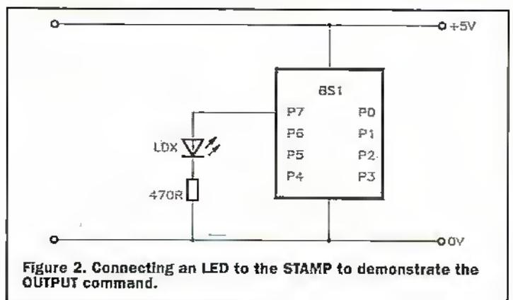
Figure 2. Connecting an LED to the STAMP to demonstrate the OUTPUT command.
