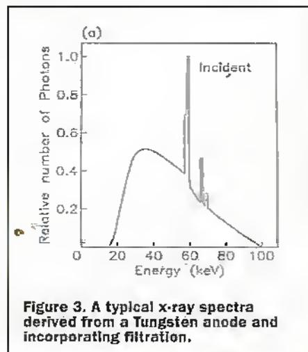
Figure 3. A typical x-ray spectra derived from a Tungsten anode and incorporating filtration.
