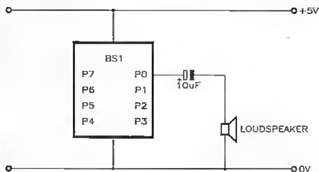
Figure 5. Connecting a loudspeaker to the STAMP to take advantage of the *SOUND* command.
