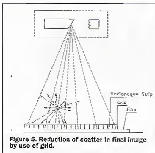
**Figure 5. Reduction of scatter in final image by use of grid.**
