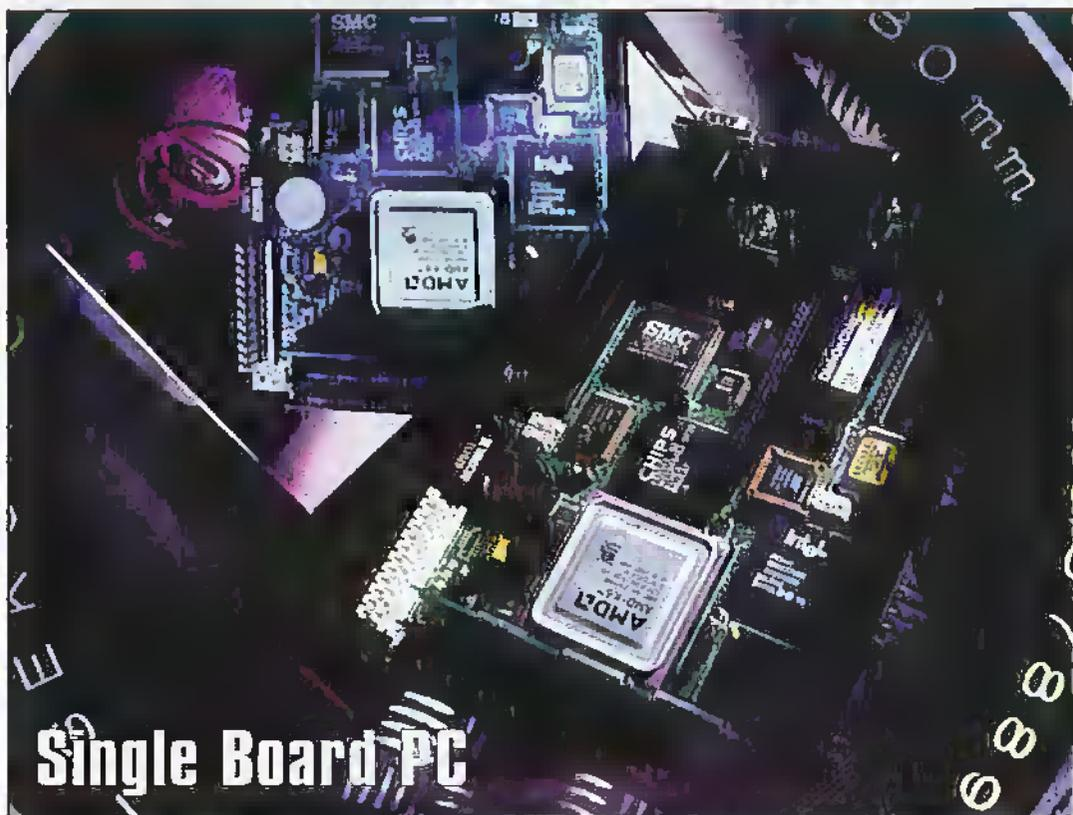
Blue Chip Technology has launched a powerful single board computer for audio, graphics and video applications. The 200MHz Pentium product has 64MB DRAM, 512KB L2 cache, an on-board SoundBlaster audio card and plug-in flash options for diskless operations.
