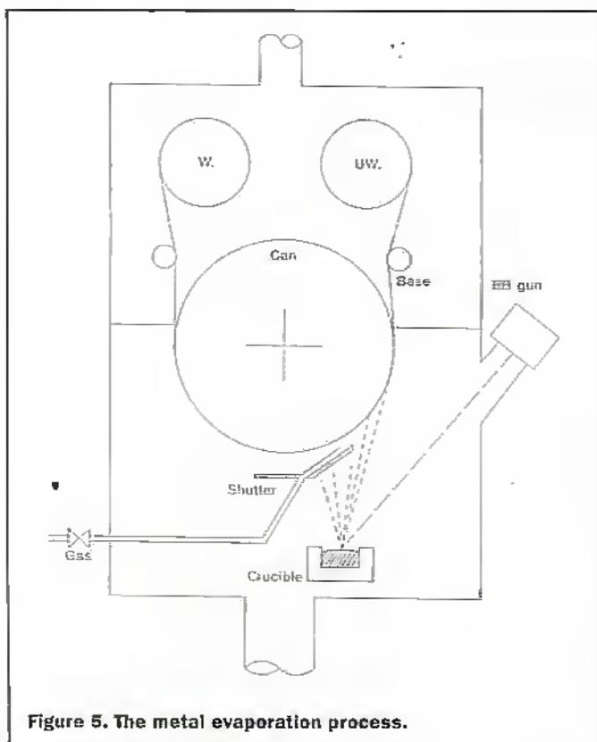
Figure 5. The metal evaporation process.
