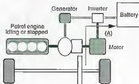
A regenerative braking used to charge battery.
