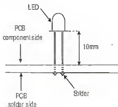
Figure 3. Mounting the LED's.
