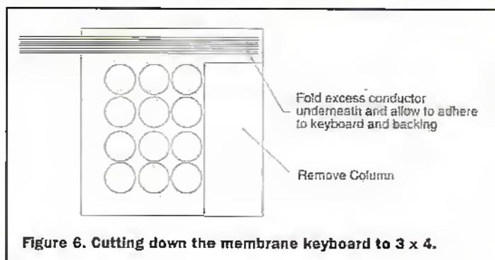
Figure 6. Cutting down the membrane keyboard to 3 x 4.
