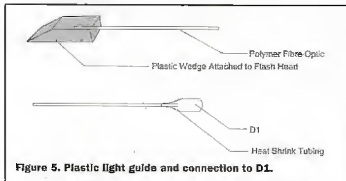
Figure 5. Plastic light guide and connection to D1.
