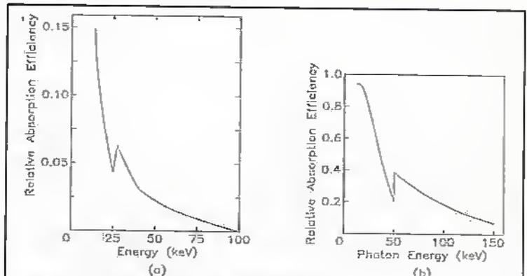
Figure 11. a) Efficiency of x-ray film alone b) efficiency of rare earth screen.
