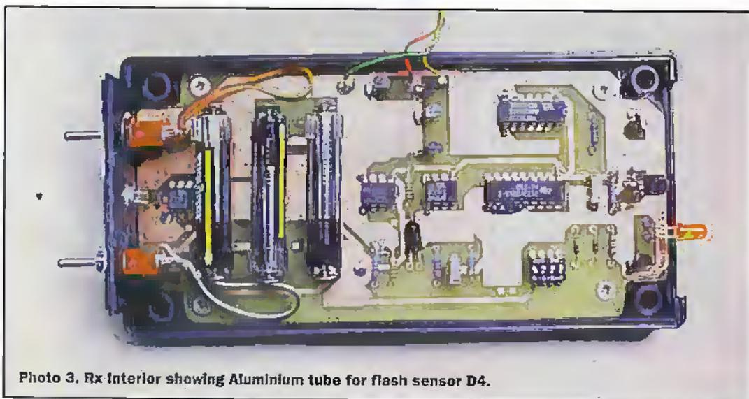
Photo 3. Rx Interior showing Aluminium tube for flash sensor D4.
