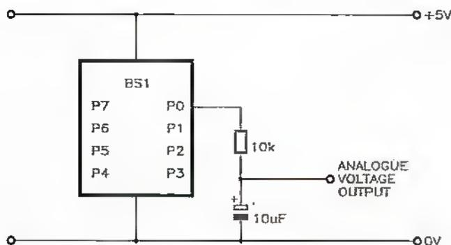
Figure 6. Configuring the STAMP for analogue output using the PWM command.
