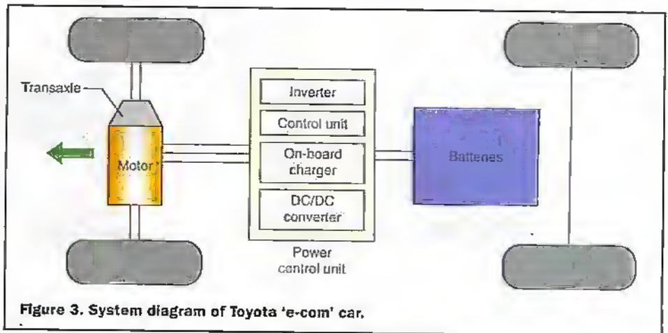
Figure 3. System diagram of Toyota 'e-com' car.
