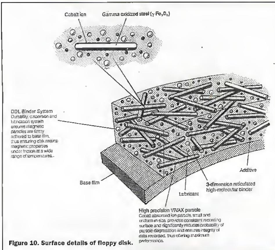
Figure 10. Surface details of floppy disk.
