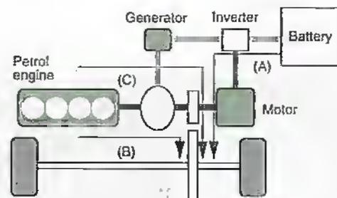
In addition to engine and generator, energy is taken from battery.
