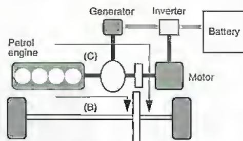
(B) Engine's power drives the vehicle and (C) generates electricity to power motor.
