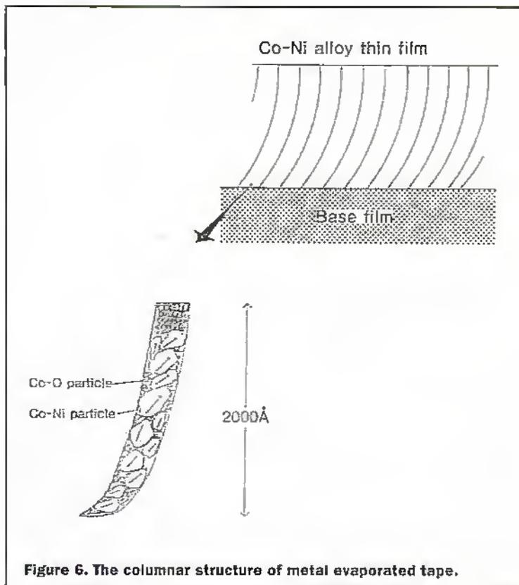
Figure 6. The columnar structure of metal evaporated tape.
