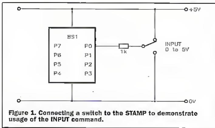
Figure 1. Connecting a switch to the STAMP to demonstrate usage of the INPUT command.
