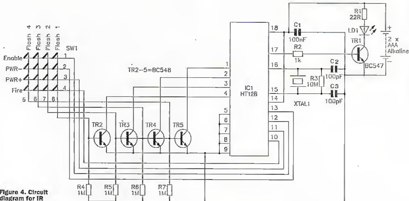
Figure 4. Circuit diagram for IR transmitter.
