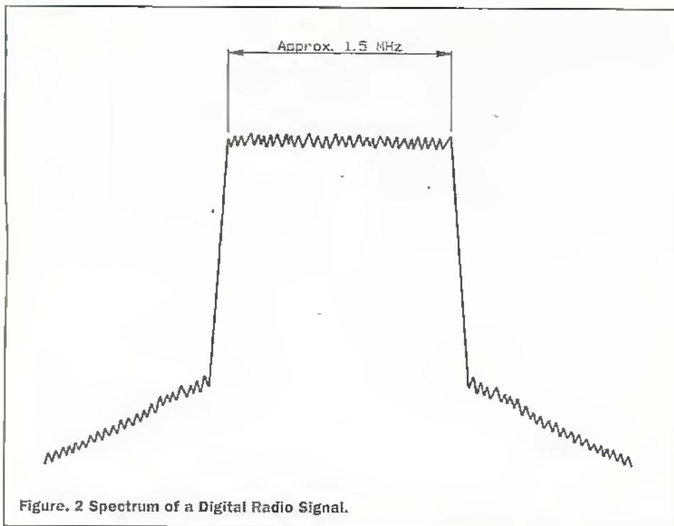
Figure 2 Spectrum of a Digital Radio Signal.
