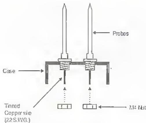
Figure 5. Fitting the probes to the case.
