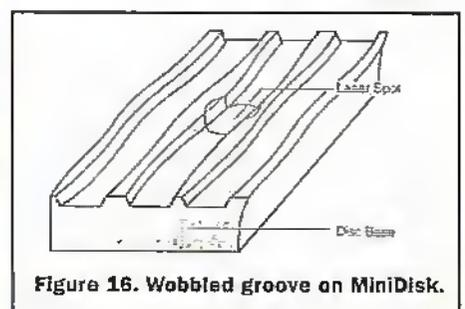
Figure 16. Wobbled groove on MiniDisc.
