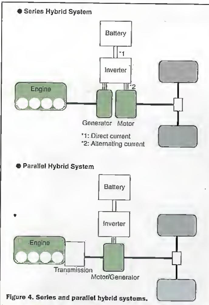
Figure 4. Series and parallel hybrid systems.
