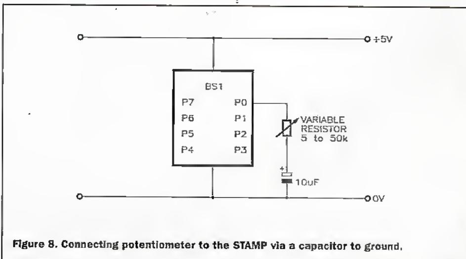
Figure 8. Connecting potentiometer to the STAMP via a capacitor to ground.
