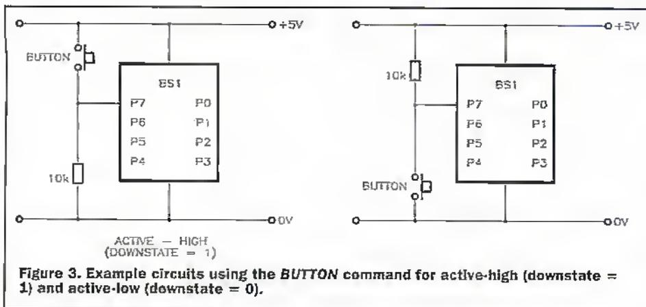
Figure 3. Example circuits using the *BUTTON* command for active-high (downstate = 1) and active-low (downstate = 0).
