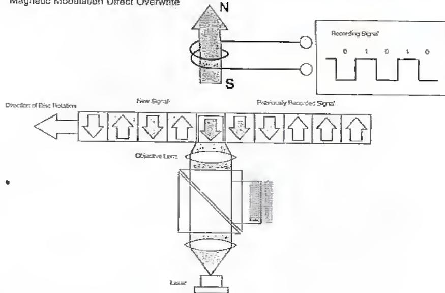
Figure 13. Writing data on a magneto-optical disk.
