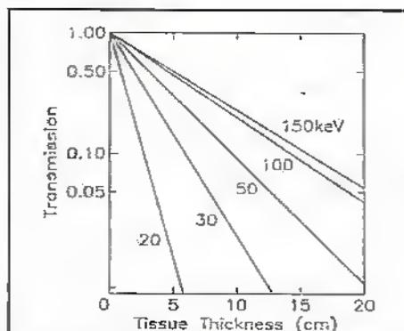
**Figure 6. Transmission characteristics of photons of specific energies appropriate for soft tissue.**
