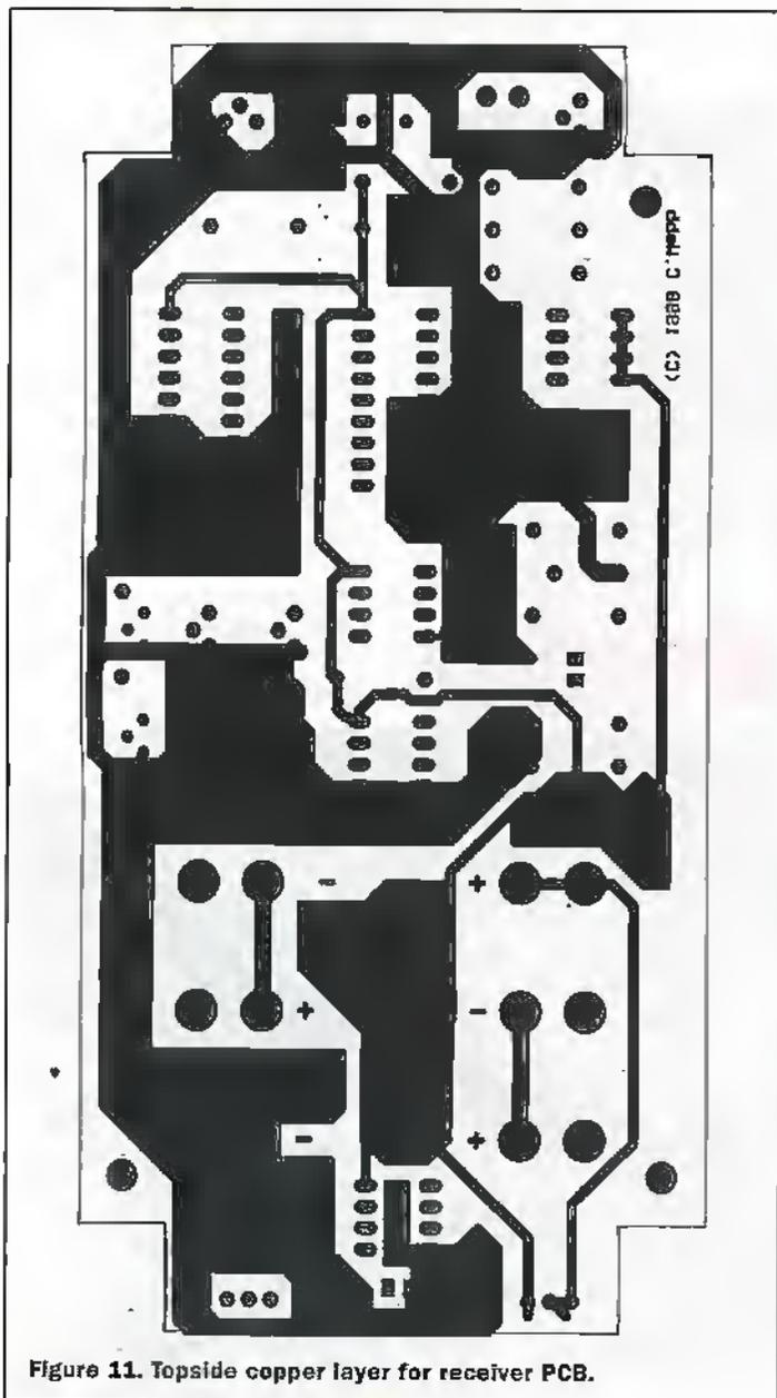
Figure 11. Topside copper layer for receiver PCB.
