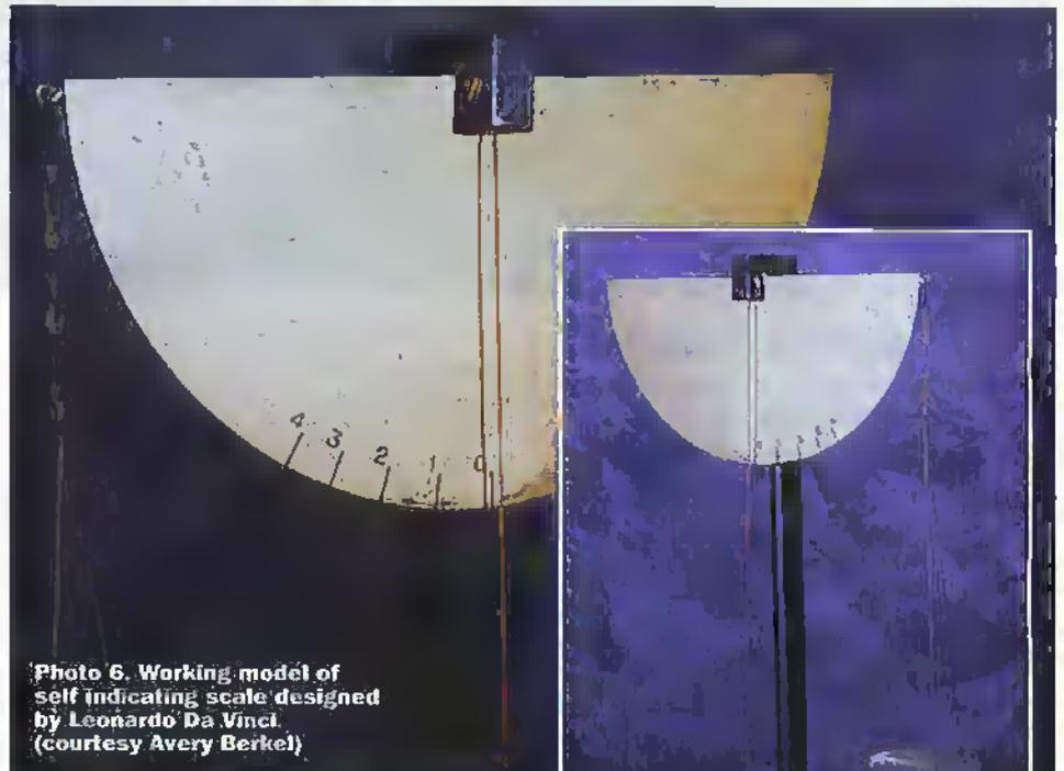
Photo 6. Working model of self indicating scale designed by Leonardo Da Vinci. (courtesy Avery/Berkel)
