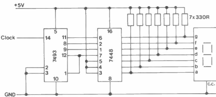
Figure 8. TTL counter with 7-segment display output.
