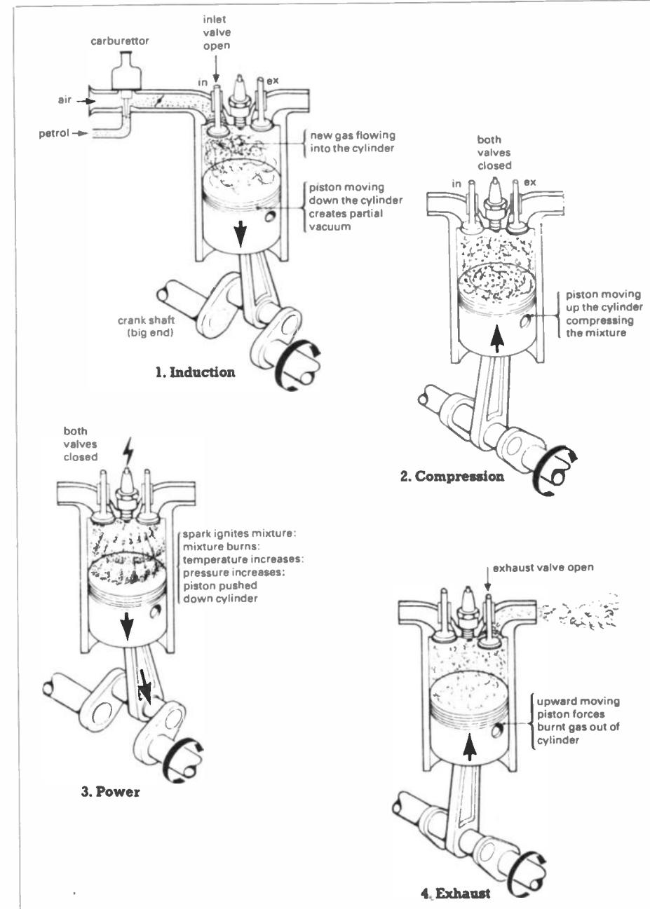
Figure 2.2. The four stages of combustion
