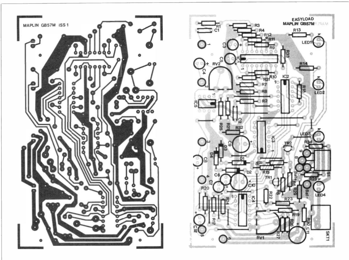
Figure 2. PCB Layout and overlay
