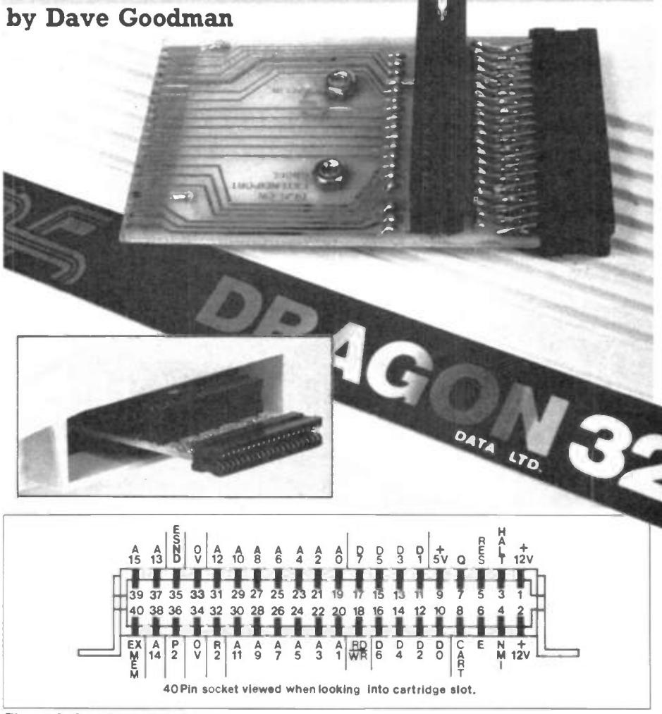
Figure 2. Cartridge slot pinouts.
