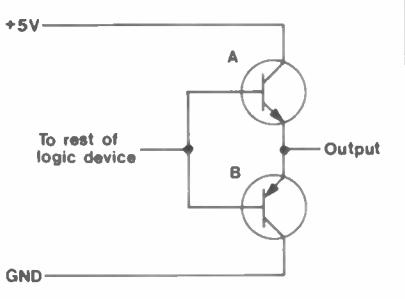
Figure 1. TTL output stage.
