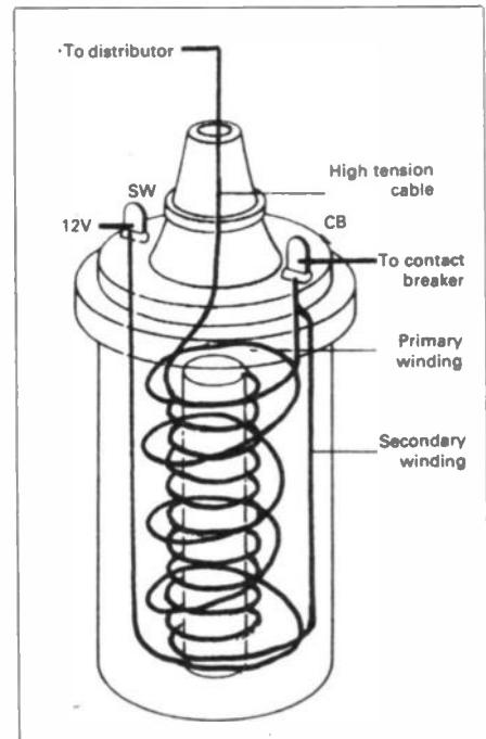
Figure 3.2. The ignition coil
