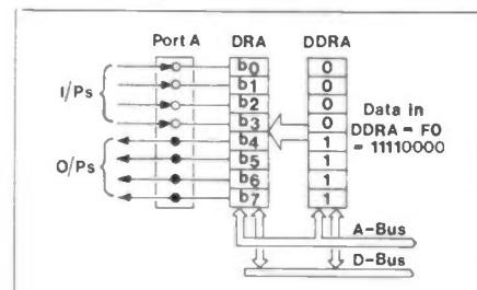
Figure 2. Configuring a Port for Input/Output Functions.
