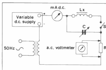
Figure 8. Turner's method for measuring large inductors.
