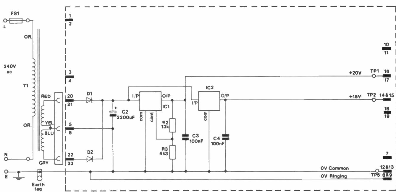
Figure 4. Modified PSU circuit
