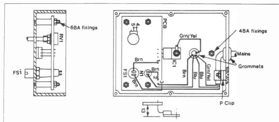
Figure 5. Assembly and wiring
