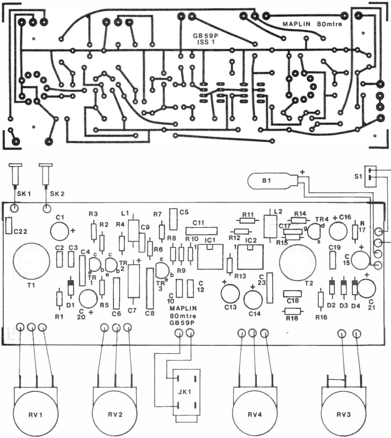
Figure 4. PCB track, legend and wiring diagram.
