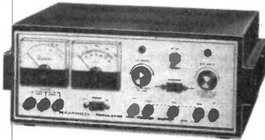
A separate transformer is used for filament voltages allowing valve filaments to be left on while the high voltage circuit is shut off. A front panel meter monitors either high voltage or bias voltage as determined by the setting of the meter switch. High voltage DC current is also monitored by a 0 to 150mA meter. A special taper control allows fine adjusting of low values of bias voltages.
