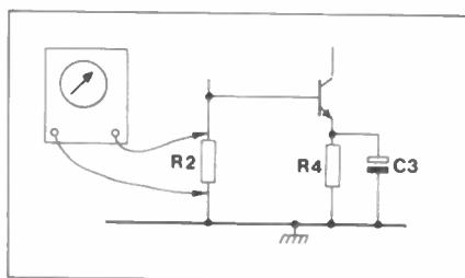
Figure 5. Measuring resistance 'in situ'.
