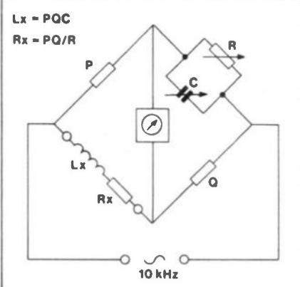
Figure 9. The Maxwell inductance bridge.
