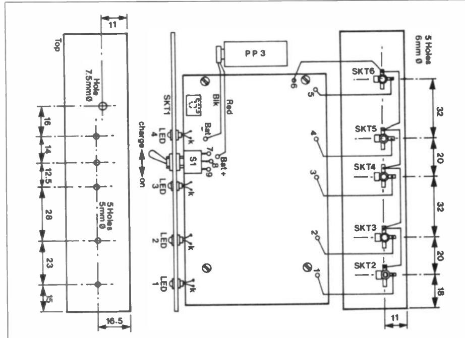
Figure 5. Box drilling
