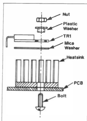
Figure 4. Mounting the transformer and heatsink
