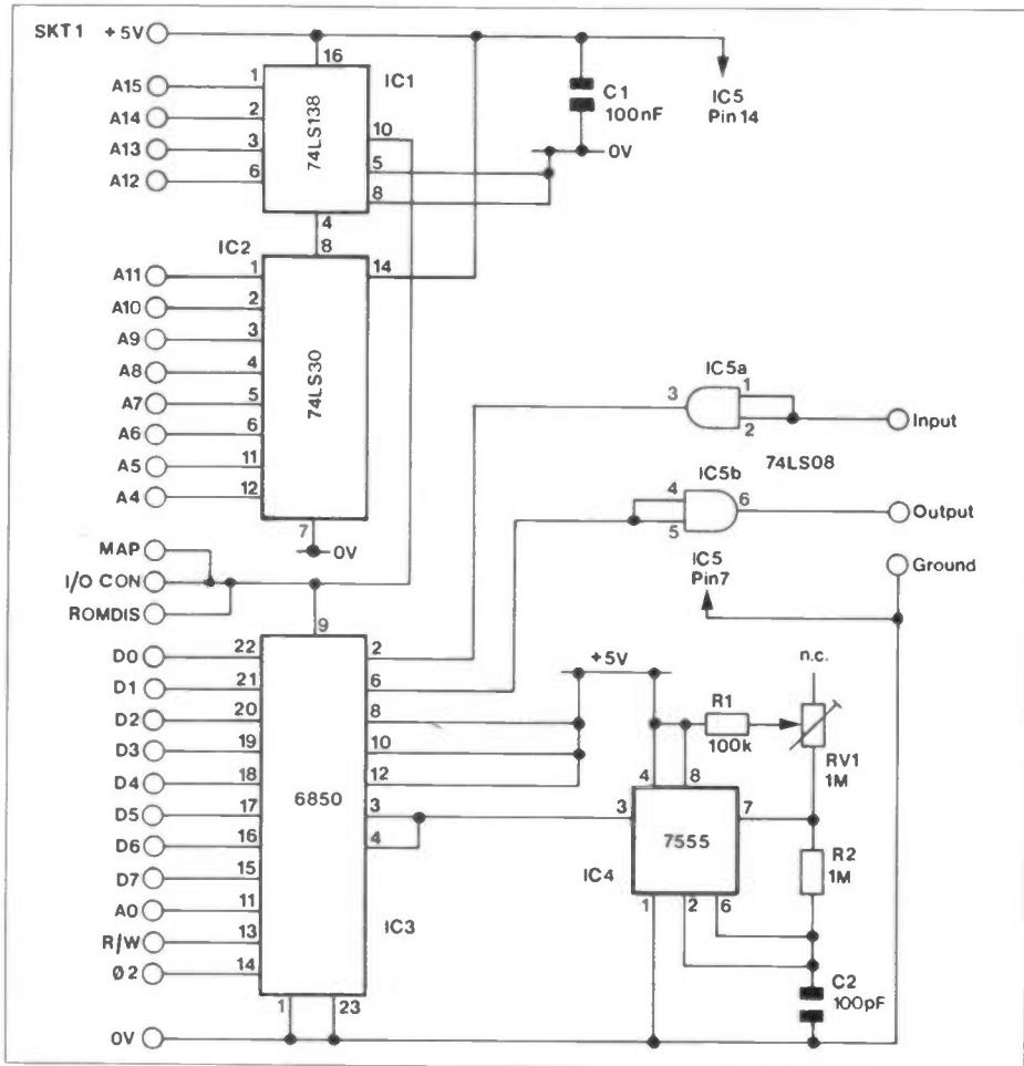
Figure 1. Circuit diagram
