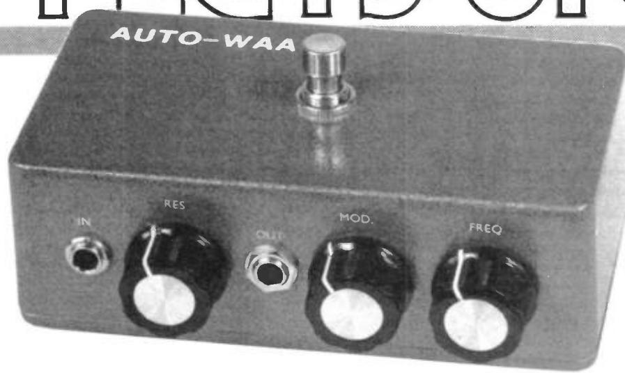
There are several ways of producing the well known and much used waa-waa effect, but in each case the basic effect is generated using some form of bandpass filter which is swept up and down over all or part of the audio band. This boosts a fairly narrow and continuously changing band of frequencies, and it is mainly the consequent variations in the relative strengths of harmonics in the processed signal that give the effect.
