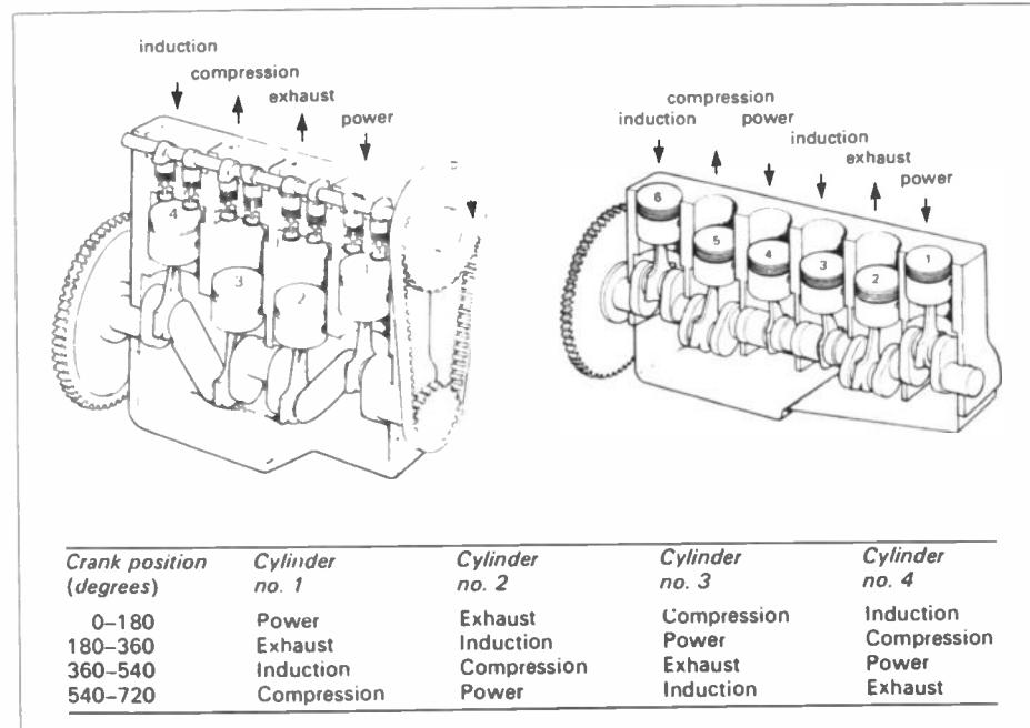
Figure 2.1. 4-cylinder and 6-cylinder engines
