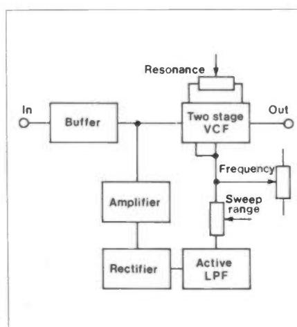
Figure 1. Block diagram
