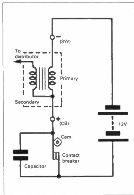
Figure 3.1. Basic high voltage generating circuit
