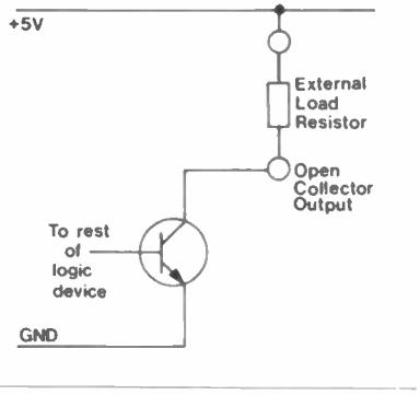
Figure 4. Open collector output stage.
