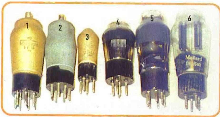
Photo 4. Valves line-up: originally 1. 6C4 octode frequency changer; 2. VP4A variable- $\mu$  pentode (damaged); 3. 2D4A double diode (damaged); 4. TT4 triode; 5. PenA4 power output pentode (failed); 6. DW4/500 full-wave rectifier.
