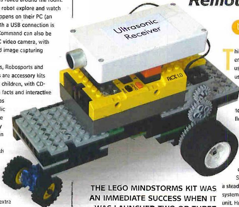
This is called the RCX unit, and it enables robots constructed using the kit to be programmed using a PC. Several programming languages can be used, including RCX code that enables the robot to be programmed via a sort of flowchart built up on the screen of the monitor. Robots can be controlled manually from the PC, programmed to 'do their own thing', or a combination of the two. Since its launch there has been
