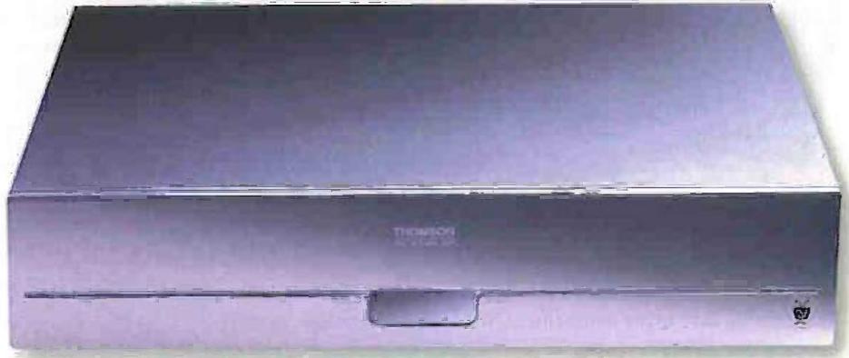
Thomson PVR10UK TiVo box, you'll find two Quantum IDE hard disks with a combined unformatted capacity of 45GB. Later models are said to have a single large-capacity drive, and a spare drive bay for adding a second drive!
