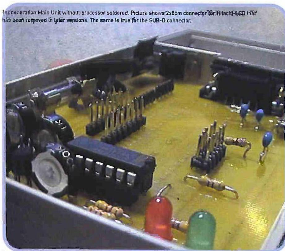
1st generation Main Unit without processor soldered. Picture shows 2x8pin connector for Hitachi-LCD that has been removed in later versions. The same is true for the SUB-D connector.
