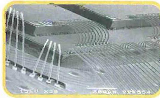
combinations that can include either wirebond or flip chip technologies within the same package.
