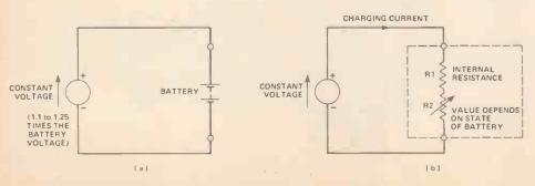
recharged, resistor R2 value is high and so the charging current is low.
