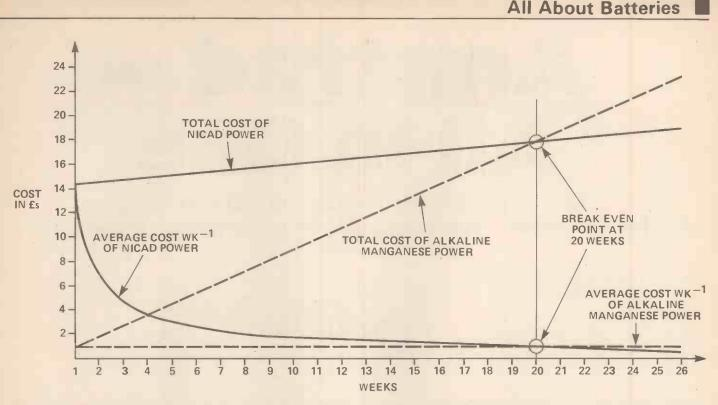
Figure 11. Comparing costs of alkaline manganese and nicad cells on a total and an average basis. Although such a comparison can only be approximate it does prove that nicad cells may be cheaper to use in the long run.
