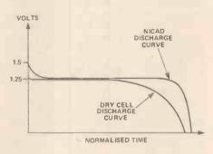
Figure 7. Graph of cell voltage against time, comparing a dry cell and a nicad cell, with a constant discharge current.
