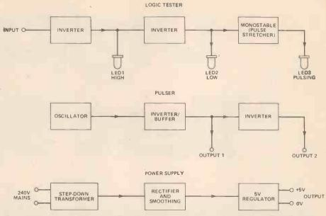
Figure 1. A block diagram of the three sections contained in the Test Set.
