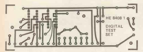
The foil pattern for the Digital Test Set. This board may easily be made using PCB transfers.
