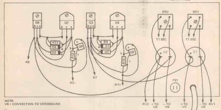
Figure 5. Wiring-up the PSU's rear panel. Take special care to orientate the electrolytic capacitors correctly. The transistors must here be insulated from the case.
