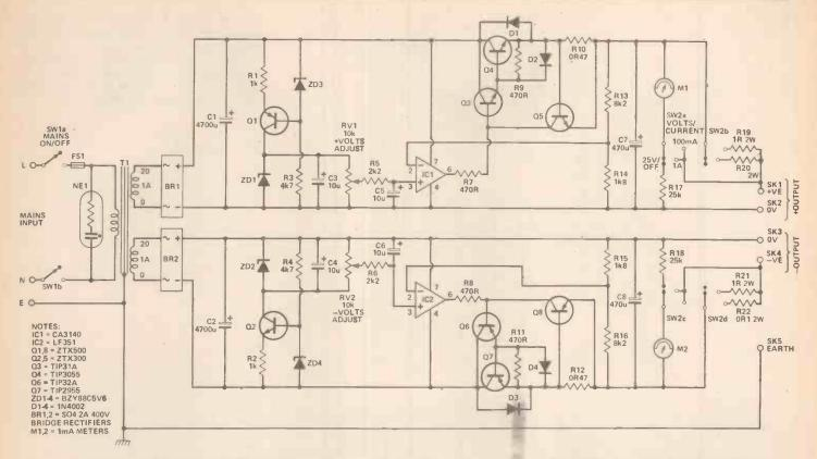
Figure 1. The Circuit, showing both positive and negative supplies.
