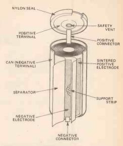
Figure 6. Make-up of a nicad cylindrical cell. The sealed vent in the cell opens at high pressures, prevent explosion due to overcharge.
