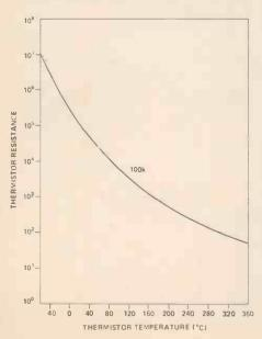
It is possible to obtain thermistors whose resistance either increases, positive temperature coefficient or decreases, negative temperature coefficient with rising temperature. For a typical negative temperature coefficient resistor, the charge in resistance with temperature is betwen thee and six per cent per degree Kelvin rise.
