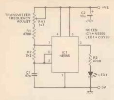
Figure 4: The Circuit of the transmitter stage.
