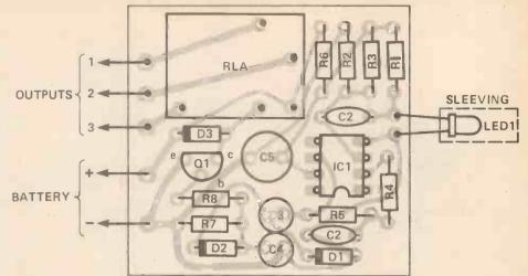
Figure 6. The PCB Overlay for the transmitter stage. Take care to orientate the electrolytics, and the IR diodes correctly, and not to mix up the transmitter and the receiver diodes.
