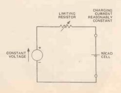
into the cell cannot exceed the maximum safe value for the cell. Generally, such a circuit must be used very carefully and under controlled conditions. Using it cells may be recharged in three main ways.
