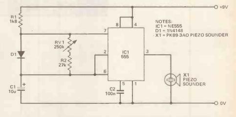
Any convenient method of construction can be used, the prototype was made using a small piece of Veroboard and a plastic box The sounder used was a PKB9-3AO from Ambit but any similar type should be just as suitable. Calibration can be any method convenient to the constructor. G. J. Hall, Leeds.
