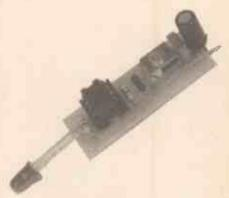
The op-amp, C1 is connected as a non-inverting AC amplifier, R2 and R3 bias the input to mid-rail. The gain of the amplifier is set by the combination of R4, R5 and C2.
