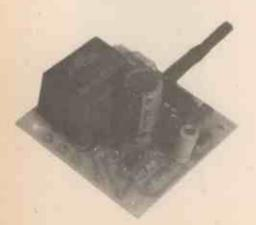
operating a relay. If the beam is broken or turned off then the receiver will detect this and release the relay. Thus any external circuit connected
