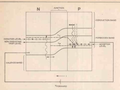
Figure 2. The PN junction of a Light Emitting Diode. When electrons jump from the conduction band to the valance band, their excess energy is converted into photons of light.
