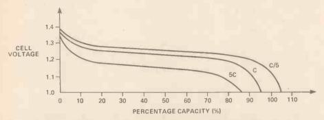
Figure 8. Showing how nicad cell capacity varies within discharge rate.
