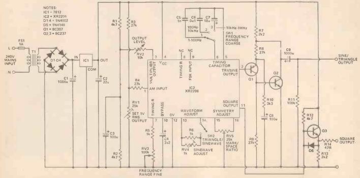
Figure 1. The Circuit. The single XR2206 function generator chip produces square and sine or triangle waves.
