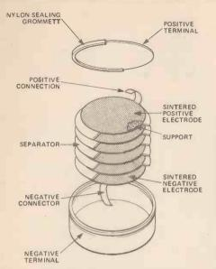
Figure 5. Make-up of a nicad button cell. Sintered electrodes allow a large surface area contact and rapid oxygen, migration between positive and negative electrodes.
