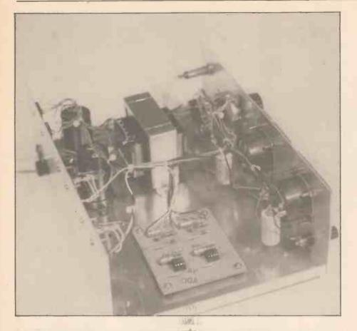
Our arrangements include the Dual PSU Tiwo 'live' views. Because of the large number of small components and trailing wires, it's important to pay a lot of attention to insulating components where necessary (as described in the text) and clipping up the wires neatly to avoid a rat's nest.
