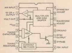
Figure 2. An internal block diagram of the XR22L6 function generator chip.
