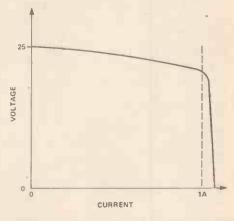
The protection offered by this circuit is not total and as such it should be remembered that if a short circuit did occur, it would be wise to remove it as soon as possible. The operation is as follows.
