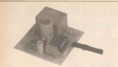
and these should be connected to the device under control, the use of changeover contacts allows you to select operation of the controlled device as a result of the beam being broken or made.
