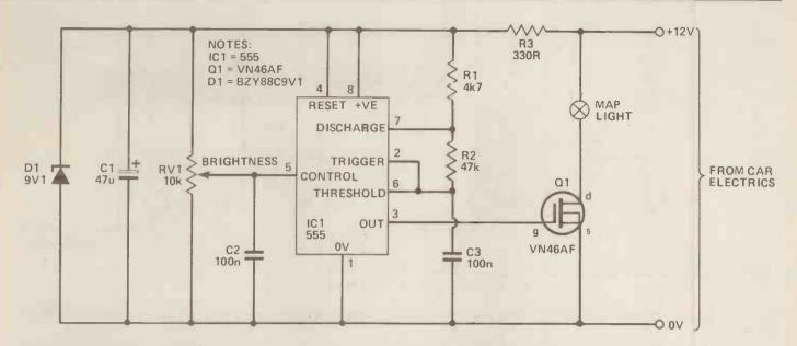
Figure 1. The circuit. The dimming is obtained by a rapid switching of the lamp, controlled by the 555 timer.
