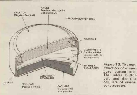
volume. Nominal cell voltage is  $1\vee35$ , and internal resistance is very stable and low.
