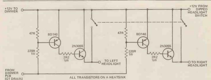
Figure 2. An experimentor's circuit for those wishing to try other applications for the circuit, including possible headlight dimming. with something which can dim
