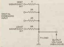
Figure 5. A binary weighted resistor network. This forms the basis of one of the simplest types of DAC.
