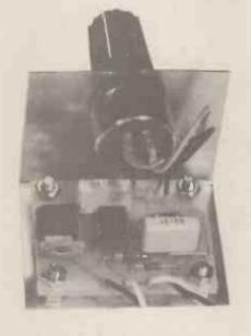
555 is not specified to get to closer to its positive supply than two volts. A ten volt Zener supply is used, so the worst case FET ON gate voltage is eight volts.
