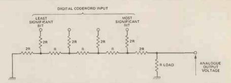
Figure 6. The R-2R resistor ladder type of DAC network.
