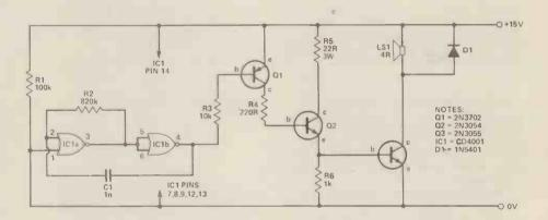
amount of heat and so should ideally be mounted on a small heatsink. Similarly, it is advisable to use heatsinks for the other two transistors.
