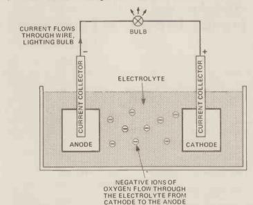
Figure 8. A basic cell in operation, in this case used to illuminate an electric light bulb.
