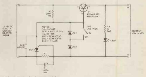
of the thyristor in the case of the large (but short) surge currents that may occur when the power supply is connected to circuits with a large capacitance across its own supply lines.
