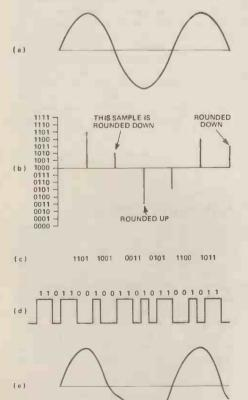
over single telephone trunks. The principle of TDM systems is repeated in Figure 2.
