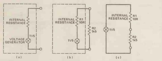
Figure 9a, b and c show the equivalent circuit (to Figure 8) of a 1V5 cell, showing internal resistance. For details see text.
