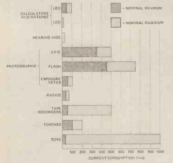
Figure 18. This graph shows the current consumption of some typical battery-powered devices. Typically, the more heat that is generated (as in the photographic flash) and the more moving parts the device has (as in the drive mechanism of a cine or tape recorder) the more expensive it is to run.
