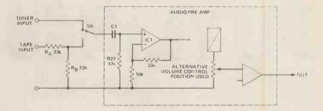
Figure 6. One possible application of the control amp: using the alternative volume control position, for recording say from a VCR and radio tuner at the same time.
