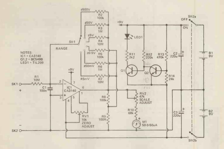
Figure 1. The circuit. All the switching is done via the six-pole switch SW1, while R10 protects the meter from overload. The red LED1 is a low battery warning indicator.
