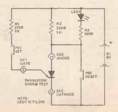
been made sufficiently low to ensure that the latching action is produced, and LED1 should remain switched on when PB1 is released.
