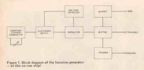
Figure 1. This gives sinewave, triangular and squarewave outputs, but the oscillator at the heart of the system is a relaxation type that produces the triangular signal.
