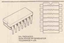
DIL Package: Compact resistor form offering considerable space savings, and very convenient for eg current limiting LED arrays, 7-segment displays, pull-up/down in logic circuits etc. Also supplied containing 13 commoned resistors.
