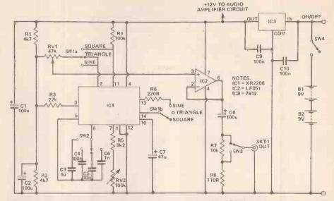
Figure 3. Circuit diagram of the signal generator section, IC1 does almost all the work, with IC2 included simply as a buffer to give a low output impedance for all three waveforms.
