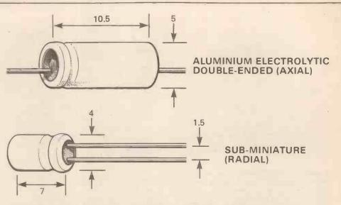
Electrolytic Capacitors: Axial electrolytics (top) are available in values up to 4700uF and at voltage ratings to 450V. Radial types, either standard of subminiature (shown at bottom), are supplied in more restricted value and voltage ranges, but take less space on a printed circuit board.
