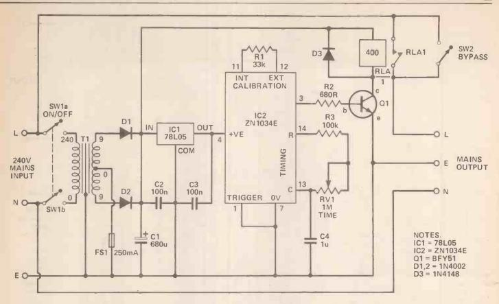
drastically, but in this case there can be a substantial change in supply stability when the relay switches on or off. A small monolithic voltage regulator, IC1 is therefore used to supply a well stabilised supply to the ZN1034E timer. The relay and driver transistor are powered from the nonstabilised supply.
