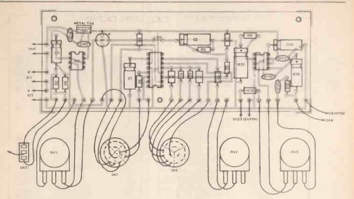
Figure 5. All components, with the exception of panel mounted controls, fit onto a single small printed circuit board (see page 64 for a full-sized foil pattern). Details of the connections from the PCB to the controls are also shown in the photographs below, and on the preceeding page.
