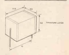
Polyester Capacitors: The box-like, silver coloured capacitors are sometimes referred to in catalogues as "Siemens" type, after the manufacturer.
