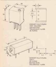
Cermet Multiturn Presets: Essential for precision adjustment. A large range of single-turn cermet trimmers are also available, eg square, vertical, horizontal and round.
