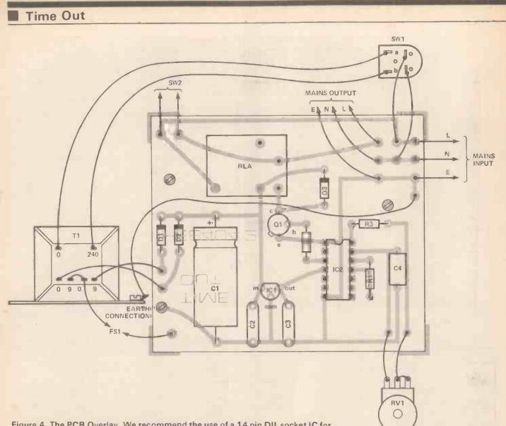
Figure 4. The PCB Overlay. We recommend the use of a 14 pin DIL socket IC for IC2. Make sure that IC1 and the semiconductors are the right way round.
