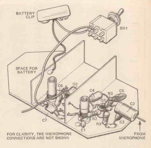
Figure 5. The construction diagram. The "up in the air" construction needs care to ensure that leads are not cut too short and that short circuits do not occur. It is not as hair-raising as it looks, however — and it is a technique worth practising.
