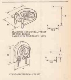
Standard Horizontal Preset (top): miniature types have pin spacings of 10.2 and 5.1mm in the same pattern.
