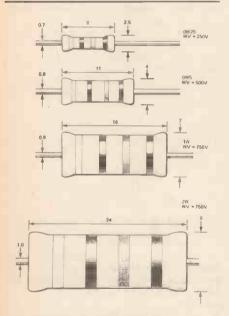
**Carbon Film: The standard** "\/4 watt 5% carbon" type, is has almost completely replaced older carbon composition resistors. Noise level is typically 1.0uV/V for any value, which is adequate for most purposes. NB: All dimensions are in millimeters.
