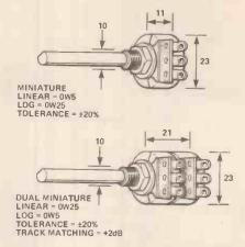
Miniature or "Midget": Carbon track potentiometers for general purpose. Dual (aka 'tandem' or 'ganged' pots) have closely matched tracks.
