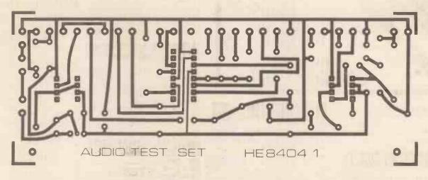
The PCB mask for the Analogue Test Set.
