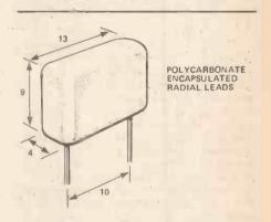
Polycarbonate: The material has better electrical characteristics than polyester and should be used, instead, in ore critical situations. A brass-encapsulated axial form is available for super-critical (eg high temperature) applications where price is of no concern!
