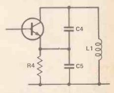
Figure 2. A diagrammatic layout of the oscillator stage.
