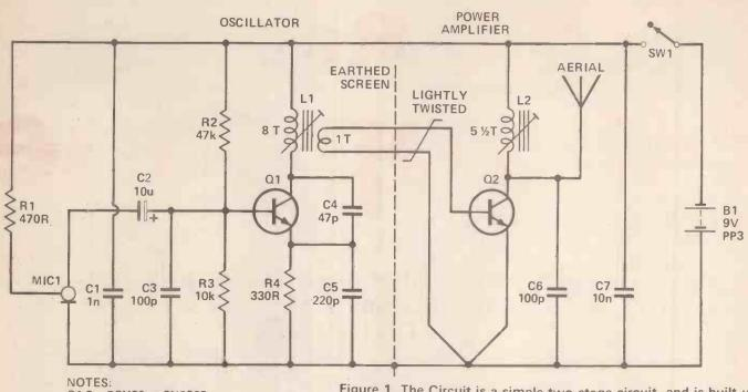
01,2 = BSX20 or 2N2369 COILS WOUND ON 3/16" DIA FORMERS FITTED WITH VHF SLUGS UNIT CONSTRUCTION ON A PIECE OF UNETCHED PCB, ON THE COPPER SIDE Figure 1. The Circuit is a simple two-stage circuit, and is built up "freehand" on a piece of unetched PCB — a common enough technique in radio, but not often seen in HE.
