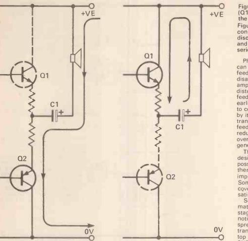
the junction of the emitters, which should be a half that of the supply, will be higher because the upper transistor is turned on harder and so has a smaller voltage drop across it.
