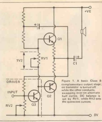
So the reduction becomes 82.5 per cent of the previous figure. It can be seen from this that the effect of variations of  $h_{FE}$  on output voltage, hence on balance between the two outputs transistors, increases withan increase in source impedance.
