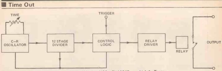
Figure 2. The block diagram shows the internal blocks of IC2, a ZN1034E, on which the Timer is based.
