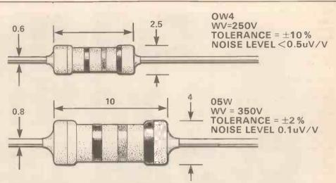
Metal Film: General purpose high stability types with low temperature coefficient. Five-band colour code gives three significant figures, multiplier and tolerance.
