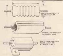
Wire wound: Silicone coated types (top) suitable for general use up to 10W rating. Ceramic encased (middle) types are useful where high insulation resistance is needed (eg mains circuits); also supplied at 4W, 7W and 11W ratings. Aluminiumclad resistors (bottom) will rarely be used by the home constructor!
