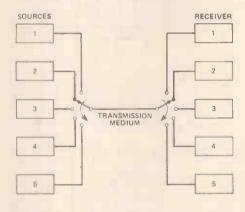
Figure 24. The principle of time division multiplexing. (TDM).
