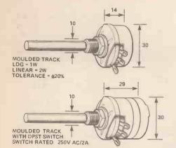
Moulded Carbon Track: The usual potentiometer chosen for panel mounting in non-critical applications. Also available with DPST switch rated for mains voltage (bottom).
