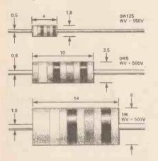
Carbon Composition: Older type resistor, for general use where temperature coefficient and tolerance not critical; noise levels generally greater than 2uV/V. Carbon comp resistors are not usually available in values below 10R.
