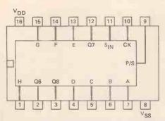
Figure 16. 4014 CMOS eight-bit shift register.
