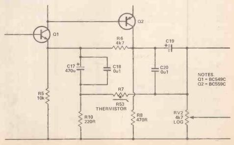
Figure 3. A different method of gain control, where R7 and LP1 are replaced with an R53 thermistor.
