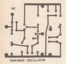
The PCB mask for the Sine Wave Generator
