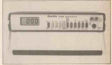
The TM356 is a battery-operated lab multimeter. With twenty nine ranges it can measure voltage from 100uV-1000V (750VAC), current from 100nA-10A and resistance from 100mR to 20MR. Battery life from alkaline 'C' cells is over 3000 hours, and a low-battery indicator shows when 10% battery life remains. The ABS case has a handle and stand for portable and bench use, and the weight is 1200gm with full batteries. The price is £85 plus VAT.
