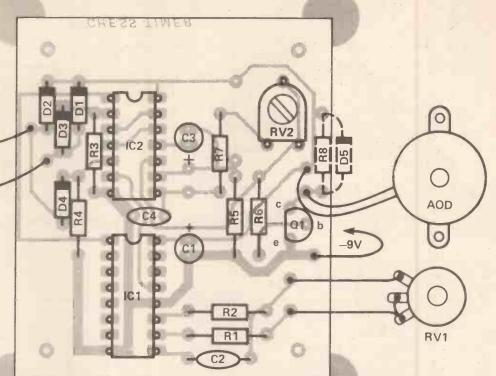
and turning on, check again for solder bridges or for components the wrong way round, and do check that the battery connections are correct. If you don't, you may need to buy some new components!
