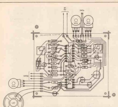
Figure 5. The PCB overlay. The long lengths of wire used to connect the switches (see photo below) make the mounting less fiddly, while not being so long as to be untidy.
