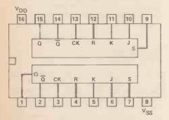
Figure 13. 4027 CMOS<sup>-</sup>dual, JK-type bistable.
