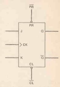
Figure 6. Circuit symbol for a JK master-slave bistable.
