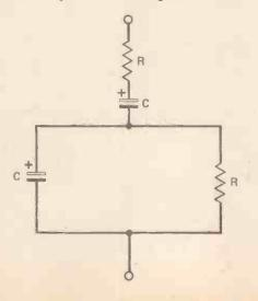
of the output. So, the gain of the amplifier must be at least three to sustain oscillation.
