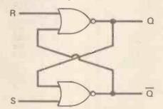
Figure 2. A simple form of electronic memory using two NOR gates — the SR-type bistable.
