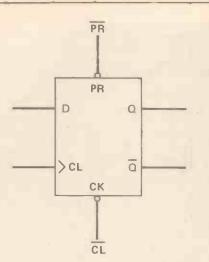
Figure 4. Circuit symbol for D-type bistable.
