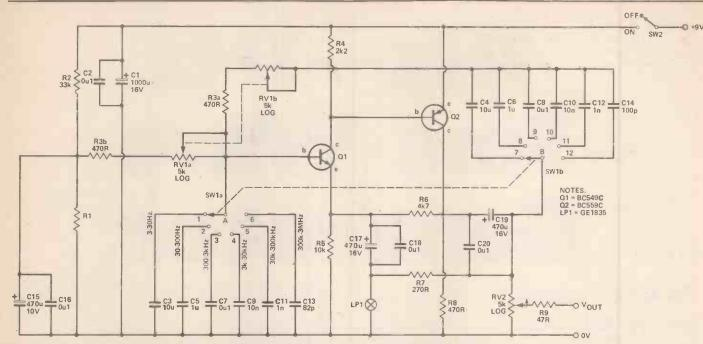
Figure 2. The Circuit. Note that R3a and R3b are two separate resistors. This diagram shows the gain controlled by a filament bulb. See also Figure 3.
