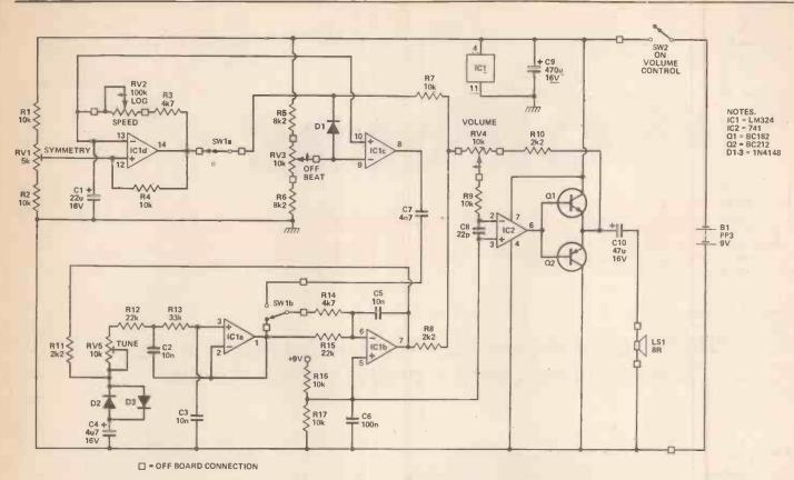
Figure 2. The circuit. The tuning oscillator also modifies the sound from the offbeat comparator.
