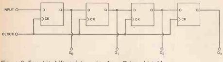
Figure 8. Four-bit shift register using four, D-type bistables.
