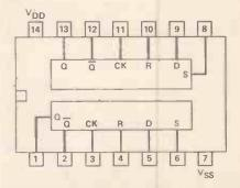
Figure 12. 4013 CMOS dual, D-type bistable.
