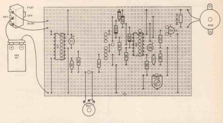
Figure 6. This Veroboard layout is untested and has been laid out without regard to size, to assist experimenters doing their own layouts. It is not the same as the Vero layout used in the original model (see picture, bottom left), which was constructed for a maximum saving on space. Also, the switch wiring in the unmodified model is different from the arrangement used in the project, so don't attempt to copy it. The Verolayout in the photo may offer some clues to anyone doing his own Veroboard.
