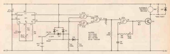
Figure 2. The circuit. R8 and D5 are optional components which may be required according to the exact method used to give the audible tone.
