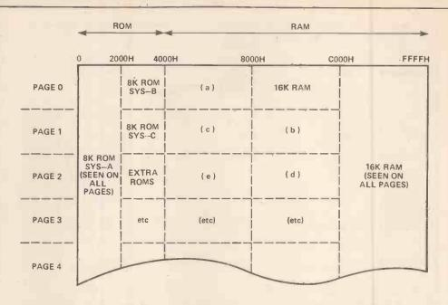
Figure 2. The MTX features a paged memory system, allowing extra ROM and RAM to be added. The diagram shows the basic MTX 500 configuration; RAM is added in the order (a), (b), (c), and so on.
