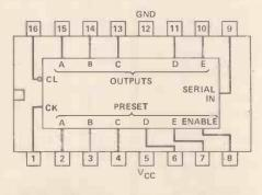
Figure 14. 7496 TTL five-bit shift register.
