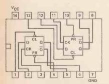
Figure 10. 7474 TTL dual, D-type bistable.
