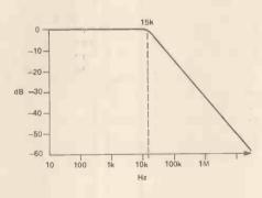
Figure 9. The frequency response of a low pass filter with a corner frequency of 15 KHz.
