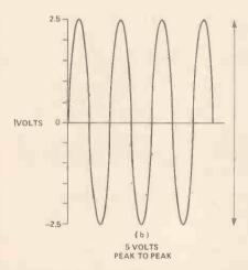
Figure 5. AC input and output voltages to and from an op amp with a gain of five.
