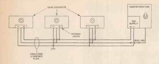
Figure 2. Connecting up a number of Quizmasters to a Master Control switch. See Figure 7 for a suggested circuit.
