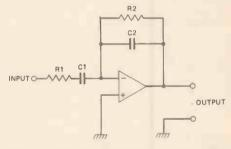
Figure 13. An amplifier bandwidth defined by an op amp with high and low pass filters.
