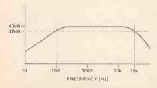
Figure 6. The frequency response of an amplifier with a bandwidth of 100Hz to 15Hz.
