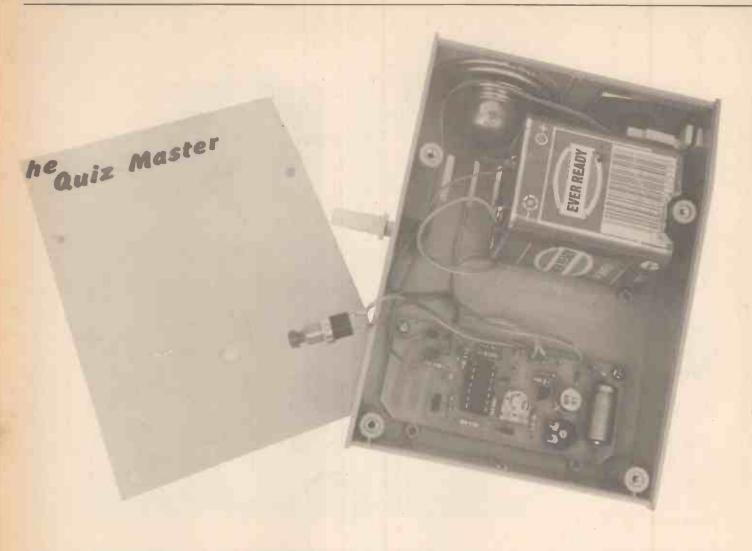
Figure 6. Internal wiring of the Quizmaster.
