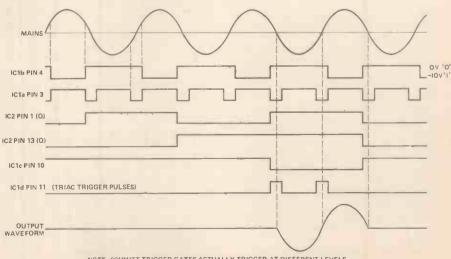
NOTE. SCHMITT TRIGGER GATES ACTUALLY TRIGGER AT DIFFERENT LEVELS, DEPENDING ON WHETHER THE INPUT(S) ARE SWINGING POSITIVE OR NEGATIV (HYSTERESIS) HOWEVER IN THE INTEREST OF CLARITY THIS DETAIL HAS NOT BEEN SHOWN.
