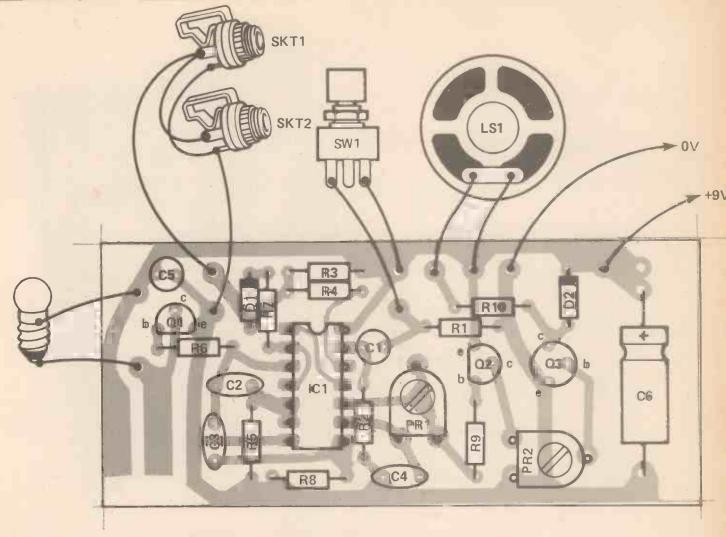
Figure 4. The Component Layout. Note the orientation of D1 and 2, C2 and IC1.
