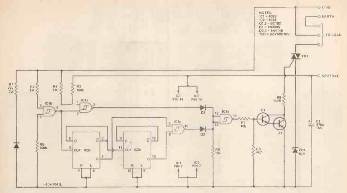
Figure 1. The circuit. The CMOS input protection diodes prevent the inputs from a possible swing to around ± 34V!
