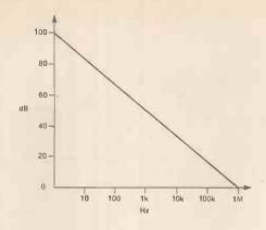
Figure 7. Open loop frequency response of a 741 op amp.
