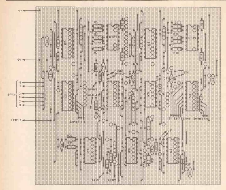
Figure 4. Veroboard component layout for intrepid experimenters; it has not been constructed and tested, and so cannot be guaranteed to work—see also the note below! Stop Press: C8, which should be connected across the DC supply rails, has been omitted.
