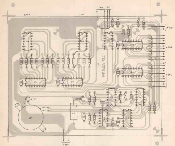
Figure 3. The PCB component overlay; most components are mounted on the board, including the piezo sounder. The power supply must be between 9V and 15V DC but does not have to be regulated.
