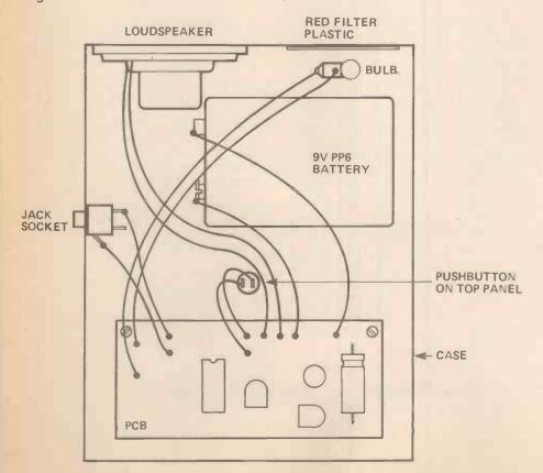
overlay diagram. Different versions may be used, but their pinouts will vary and should be checked before soldering.
