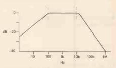
Figure 12. The frequency response of cascaded high pass and low pass filters with corner frequencies of 100 and 15KHz.
