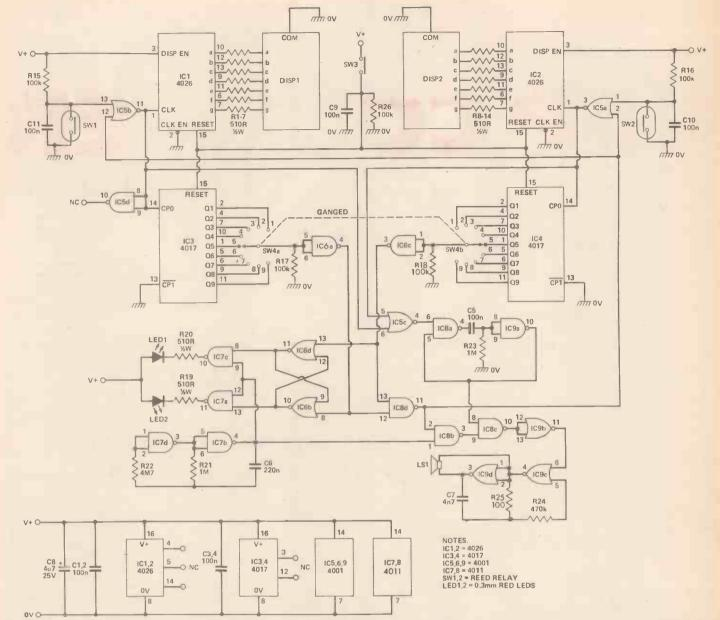
Figure 1. The circuit of the Lap Counter comprises two identical counting and display blocks, together with the win detection and indicator circuits, below.
