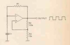
Figure 22. A squarewave generator using an op amp with negative and positive feedback.
