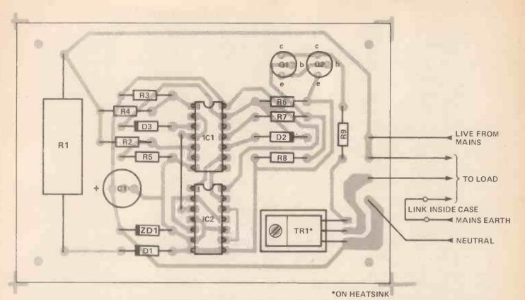
Figure 3. The component layout. Build and test the power supply section first, checking that R1, C2, D1 and ZD1 are the right way round.
