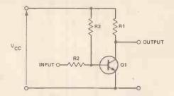
Figure 19. AC current amplifier formed by a single transistor.
