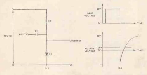
Figure 16a) Resistor/capacitor/diode (RCD) circuit b) Operating voltages of the RCD circuit.
