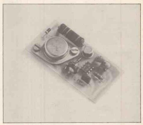
required in this supply path to stop the switching transistor initially shorting to ground through the park switch (D3, in the complete circuit diagram). Both the switching transistor and the diode must have high power ratings because the transistor must handle the motor starting surge current while the diode carries the motor current for most of the "wipe".
