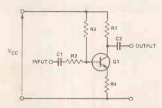
Figure 21. Common emitter amplifier with feedback and DB blocking capacitors.
