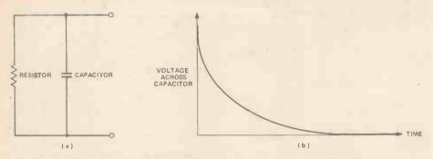
Figure 14. Discharging a charged capacitor through a parallel resistor.
