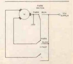
Figure 1. The wiper control circuit shown is conventional on most makes. The Delay unit is installed in the 'slow speed' circuit, but slow wipe is still possible by turning the delay to zero.
