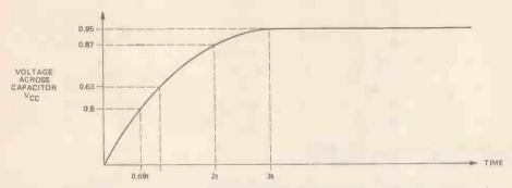
Figure 15. Important points on the exponential curve of a charging capacitor.
