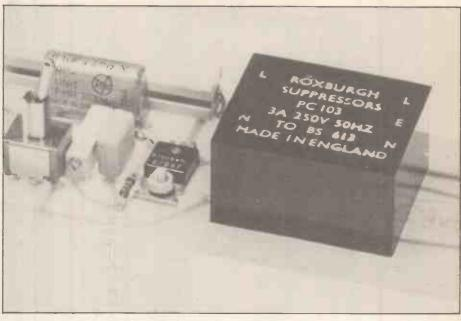
suitable for protecting a wide range of equipment from mains transients and interference. Rifa self healing capacitors ensure reliability and the units are fully encapsulated for complete environmental protection. The photograph shows the PC 103 mounted on a mains input board.
