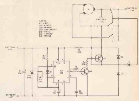
Figure 2. The circuit uses a 555 timer in the astable mode to provide the delay function. The unit is connected into the slow speed wiper circuit at the points indicated by the breaks.
