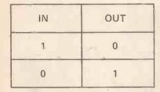
Figure 5. Truth table of an inverter gate.
