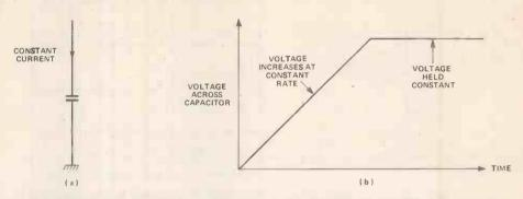
Figure 12. a) A constant current used to charge a capacitor b) Capacitor voltage when a constant current is applied then removed.
