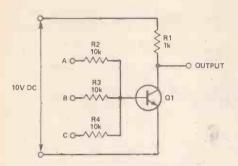
Figure 6. A single transistor, threeinput NOR gate.
