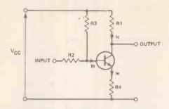
Figure 20. Common emitter amplifier with feedback.
