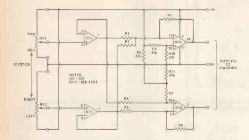
THIS mixer was designed to be fitted to a radio control transmitter to allow a tracked vehicle (eg a tank) to be controlled from a resistive joystick controller.
