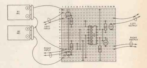
Figure 2. Careful use of screened cables for all inputs and outputs when constructing the Veroboard will keep undue noise out of the system.
