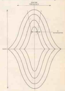
Figure 3. This graph shows a few of the infinite variety of response curves that the Para-Q can generate. There are three variables: the centre frequency can be positioned anywhere between 50Hz and 11kHz; the gain at that frequency can be varied by ±20dB; and the Q or bandwidth of frequencies effected can range from 1 to 25, giving boost or cut over a very narrow range or over a wide band of frequencies.
