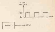
Figure 17. Block diagram of an astable.
