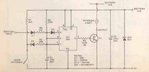
Figure 1. The circuit is based on a 555 used as a comparator.
