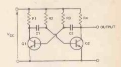
Figure 18. Astable formed by two transistors and two RCD circuits. The diodes of each RCD circuit are formed by the base-emitter junction of the transistors.
