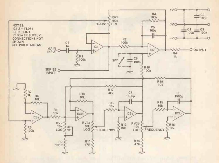
Figure 1. The circuit shown above is for one channel of the stereo pair. Switch SW1 is an optional bypass for the channel; several other modifications which alter the characteristics of the equaliser are described in the text.
