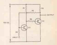
Figure 9. A two-transistor bistable formed by connecting the output of the first to the input of the second.
