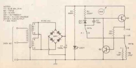
Figure 1. The values for current limiting resistors R4 and R5, must be calculated from the formula given in the text.
