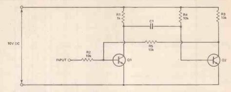
Figure 11. Monostable formed by two transistors connected by a capacitor.
