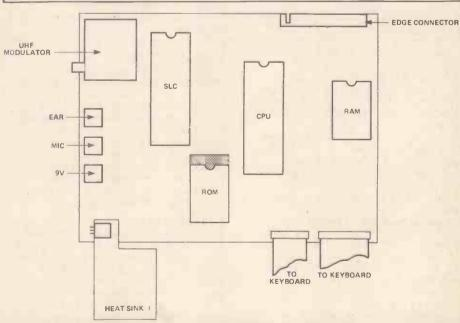
Figure 4. The component layout inside the ZX81. The 24-pin ROM is mounted in a 28-pin socket; the hatched area indicates the unused pins.
