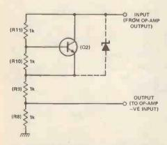
Figure 5. The operation of the 'Zener' network when the input voltage is positive.
