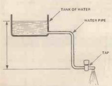
Figure 2. Simple domestic water system. The water tank is at a height, h, above the tap.
