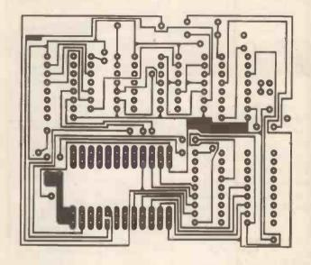
The printed circuit for the ZX81 High Resolution Graphics Project uses a double-sided board; on the left is the foil patter for the component side and on the right is the bottom foil pattern. The PCB supplied by Cambridge Computing will be a through-hole-plated type, but home constructors will need to solder links to connect the top and bottom tracks. Do this very carefully as faults, especially dry joints, can be extremely difficult to locatel
