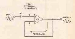
Figure 1. Block diagram of the op-amp unit.
