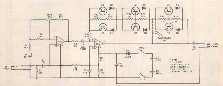
Figure 1. The circuit, with an optional third stafe for experimenters. For other constructors, the third-stage is by-passed by a wire link.
