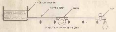
Figure 3. How a water pump can be used to create a pressure difference and cause water to flow along a pipe.
