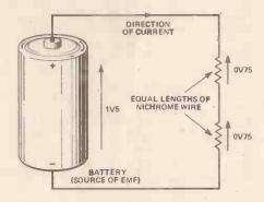
Figure 6. The battery, as a source of EMF, creates a current which in turn causes potential differences to occur across the two lengths of nichrome wire.
