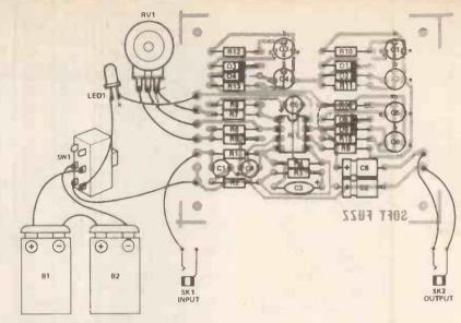
Figure 8. The PCB overlay.
