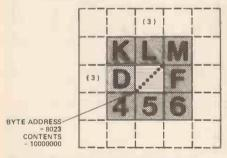
Figure 7. Illustrating the display method for graph plotting. The character ('E' in this example) is replaced by a dot pattern corresponding to the line segment to be plotted. Extended plots can be formed by joining line segments.
