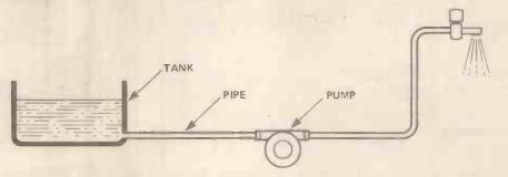
Figure 4. A water pump can also make water flow upwards, against gravity.
