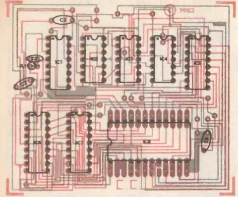
Figure 3. The double-sided, through-hole-plated PCB and component overlay. Readers making up a board themselves will need to wire through-links to connect the two sides of the printed circuit.
