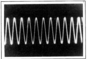
Figure 6. A 50 Hz waveform produced by touching the input of a 'scope.
