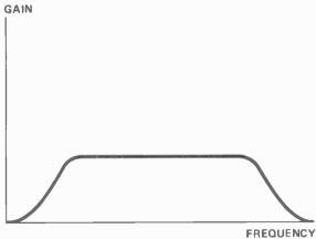
Figure 3. Reducing frequency distortion by negative feedback; (a) Graph of gain plotted egainst frequency for an amplifier without feedback; (b) the effect of negative feedback is to reduce the gain, creating a flat portion of graph.
