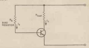
Figure 8.11 A single-resistor bias circuit.
