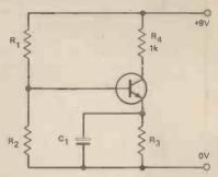
Figure 8.15 The potential divider bias system; C1 is short circuit for AC signals.
