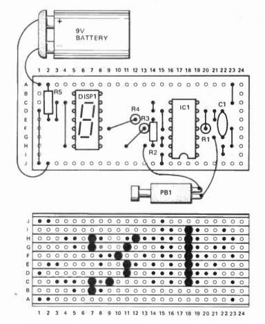
Figure 2. Veroboard layout of the project, showing component locations and track breaks underneath the board
