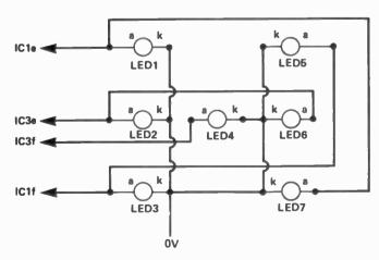
Figure 4. Connection diagram for the LED's.
