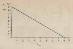
Figure 8.5 A graph of collector voltage plotted against collector current for a transistor with a load resistor, when the base current is varied.
