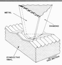
RCA's Selectavision system uses a metal diamond composite stylus running in modulated grooves on the disc. The stylus tip is only S  $\mu m$  by 2  $\mu m$  and the groove pitch is 2.6  $\mu m$ . Wear is said to be its biggest problem.
