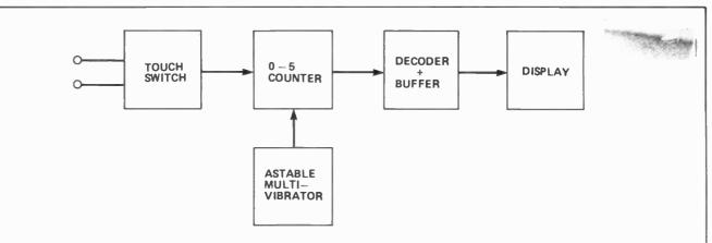
Like nearly all electronic circuits, this one may be understood if it is broken down into small blocks. This is called 'partitioning' and it is a technique used, for example, by engineers to test circuits bit by bit. From the block diagram it can be seen that there are five distinct blocks in the Digital Dice project.
