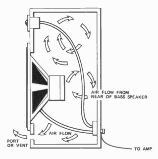
the principles, but as they are largely irrelevant to how a speaker sounds, we are not going to spend too much time on the differences here. Bass reflex enclosures are more efficient than the others, but at the cost of bass output. Transmission lines give the best bass response of the three, but at the cost of larger enclosures.
