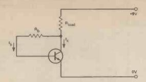
Figure 8.13 The negative-feedback bias system.
