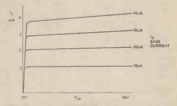
Figure 8.3 The family of graphs which is obtained when collector current is plotted against collector voltage for several different values of base current.
