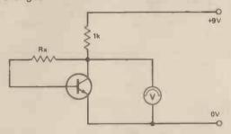
Figure 8.14 The negative feedback bias system in action; the HE Meter is set to its 10 V range. Suitable values for Rx lie between 68k and 100k.
