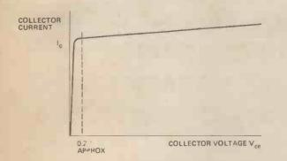
Figure 8.2 The effect of collector voltage on the collector current when the amount of base current is fixed. This graph is called a "characteristic curve" because it is peculiar to (ie characteristic of) a particular transistor.
