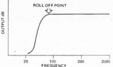
Figure 1. Typical bass response of a speaker system.
