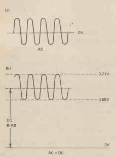
Figure 8.9 AC (a) compared to the mixture of AC and DC (b) which is needed at the input of a transistor amplifier.
