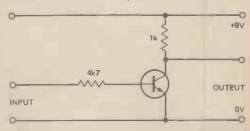
Figure 8.8 A switching circuit. The resistor in series with the base is essential to prevent excessive base current.
