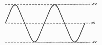
Figure 1. Voltage emplitude. This wave has a voltage emplitude of 4 V peak-to-peak.
