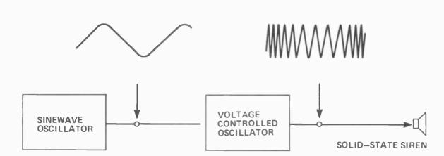
A low frequency (about 2 Hz) oscillator provides a sinewave control voltage. for a voltage controlled oscillator (VCO). Thus the VCO output frequency varies, up and down, at a rate of 2 Hz (ie, twice a second). The resultant output is used to switch on and off a solid-state audible warning device to produce a sound effect similar to American police car sirens.
