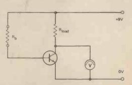
Figure 8.12 Trying out a single-resistor bias circuit. Set the HE Meter to its 10V range and try different values for Rb, starting with 100k.
