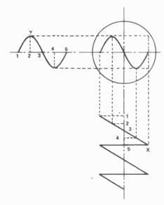
Figure 3. The deflection waveforms, applied to the X and Y plates, cause the electron beam to sweep out a faithful replica of the Y-input waveform.
