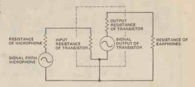
Figure 8.18 Equivalent circuit of a common-emitter amplifier 'gain block' (shown within dotted lines) with a source (microphone) and a load (headphones) connected. The total gain is reduced below that of the gain block itself because the voltage delivered by the microphone is 'loaded' by the input resistance of the amplifier. Similarly, the voltage delivered to the load is reduced because of the output resistance of the amplifier.
