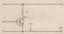
Figure 8.4 A resistor (the load resistor) connected into the collector circuit of a transistor.
