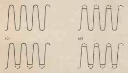
Figure 8.10 Distortion of a sinewave caused by incorrect bias or excessive signal ampliftude: (a) perfect sinewave; (b) clipped at the top (faulty bias — DC base current too low); (c) clipped at the bottom (faulty bias — DC base current too high); (d) clipped top and bottom (bias correct but signal ampliftude too high).
