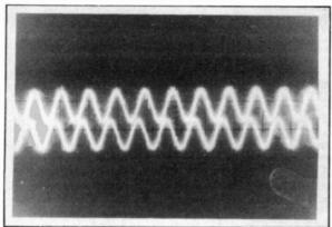
Figure 8. Comparing waveforms on a double-beam 'scope: (a) Sinewaves in phase: (b) Sinewaves out of phase.
