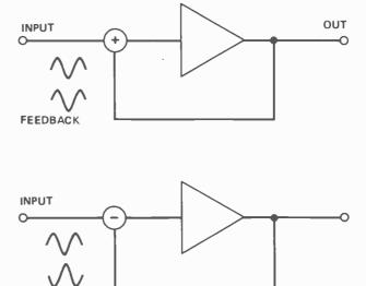
Figure 2. Feedback; (a) in phase, adding to the signal at the input (positive feedback); (b) in entiphase, subtrecting from the signal et the input (negative feedbeck).
