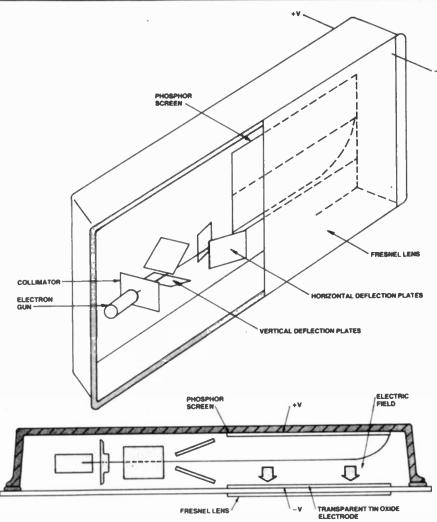
Figure 1. General construction (simplified) of the Sinclair miniature flat screen picture tube (see also picture over the page).
