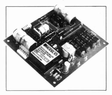
Figure 3. A typical crossover circuit. In this case the unit is the ETI V3 DIY loudspeaker which uses the three units (two of which are domed units) which provide a better spread, or dispersion of sound, than a normal cone.
