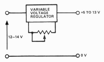
Integrated circuit IC1 is a fixed-voltage regulator which develops and holds the output voltage at 5 VDC. A typical circuit using the IC would have its common connection directly connected to the earth rail (0 V). The IC's output, in such a circuit, is at a voltage of exactly 5 V above earth. However in our circuit, a preset resistor RV1 is connected between the common connection and earth.
