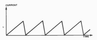
Figure 5. Because the scanning of lines on the picture tube is repetitive the current waveform is a continuous stream of sawtooth waveforms such as those shown in Fig.4. This is the picture you would expect to see on an oscilloscope connected to each coil in turn
