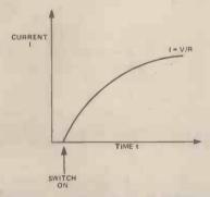
Figure 5. How the current in the circuit in Fig.4 changes after switching on
