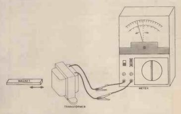
Figure 3. Inducing a voltage in a coil by moving a magnet close to it. Here one of the windings of a transformer (an iron-cored choke could also be used) connected to the HE Multitester (10 VDC range)
