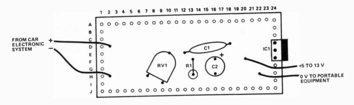
Figure 2. Veroboard layout, showing component locations along with connection details of the project. Note that there are no track breaks to make
