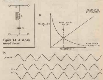
Figure 15. Reactance, voltage and current: a) how reactances of a coil and of a capacitor vary as the frequency of the signal is varied, b) voltage and current waveforms for a coil and capacitor in series at the resonant frequency of signal
