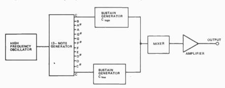
The high frequency oscillator is formed around a 555 timer, IC1. Preset resistor RV1 is a pitch control. The output of the 555 is directly coupled to the clock input of IC2, an MO83, 13-note generator, which divides down the high frequency signal in a musical ratio. The 13 outputs of IC2 form an oc-
