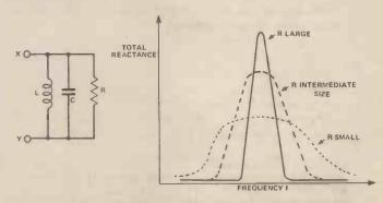
Figure 21. Effect of taking current from a resonant circuit. Adding resistance to take current causes the curve to flatten out. This is called 'damping'
