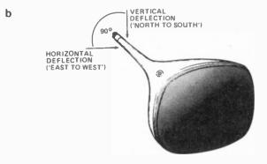
Figure 3. Position of deflection coils on neck of a TV picture tube:
