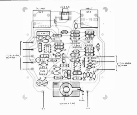
Figure 2. Component overlay of the main component PCB
