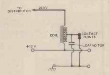
Figure 7. The traditional type of car ignition circuit. The back EMF that is generated when the contact points open is stepped up to 25 000 V (25 kV) by the coil (acting as an autotransformer, described in this article)
