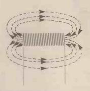
Figure 2. Shape of the magnetism when a wire is wound into a coil and current passes. This is the same shape as we would detect from a bar-shaped permanent magnet
