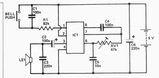
Figure 1. Circuit of the HF Doorchime
