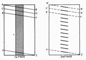
Figure 1. Transferring an image accurately from one sheet of paper to another. Light and dark areas on the first sheet are 'scanned' with a pointer and this information is transferred with a pen, line by line, to the second sheet. The pen must move in exact step with the pointer and only delivers ink to the page when the pointer is scanning dark areas. Complicated? A similar, electronic, process is used to transfer images viewed by a TV camera to the picture tube in your TV receiver
