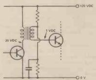
Figure 9. Using a transformer to connect signal from the collector of one transistor at 20 VDC to the base of another transistor at 1 VDC
