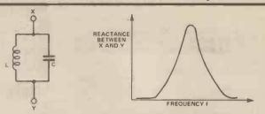
Figure 19. Parallel-tuned circuit. The reactance varies as the frequency of signal across the circuit is changed, and becomes a high value of resistance at the resonant frequency
