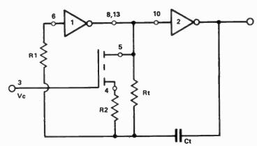
Figure 2. Voltage controlled oscillator using CMOS inverters and a CMOS field-affect transistor. Pin numbers relate to the 4007 integrated circuit. Supply connections are not shown
