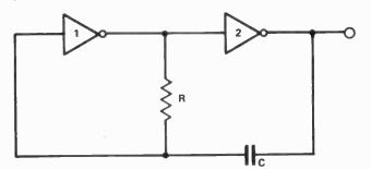
Figure 1. Simple CMOS astable multivibrator
