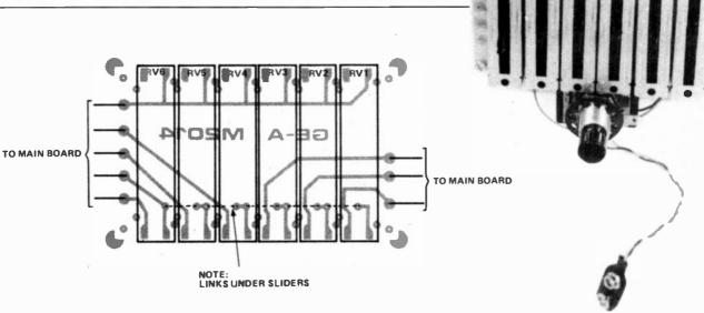
Figure 3. Component overlay of the slider PCB
