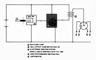
Figure 3. Siemens' integrated ignition controller used with a Halleffect ignition system
