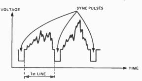
Figure 7. Waveform of signal transmitted from the studio to your TV receiver. It contains two kinds of information: regular 'sync' pulses which lock the horizontal and vertical deflection timebase circuits precisely to those in the camera, and voltage variations corresponding to the brightness information from the scene in front c, the camera lens, transmitted line-by-line
