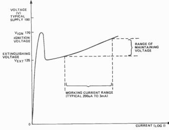
Figure 8. Typical electrical characteristic of a gas discharge display
