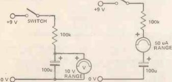
Figure 15. How to measure the voltage across a charging capacitor — this is possible only if the capacitor has a large value, because smaller values will have completed charging before the meter has had time to respond Figure 16. Circuit for measuring charge — and leakage — currents
