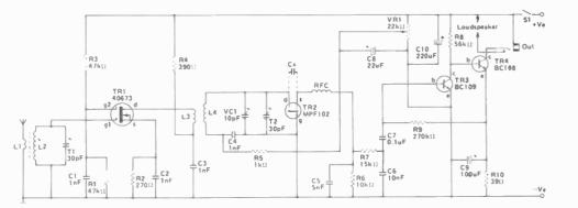
Figure 11.1 Circuit of the VHF receiver
