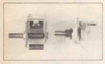
Figure 9. Variable capacitors: (a) miniature air-spaced type, (b) standard size air-spaced, (c) twin-ganged air-spaced capacitor: the two capacitors are on the same shaft so that their values change together, (d) a solid-dielectric variable capacitor — the material between the plates is a solid insulator
