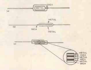
Figure 5.Mica capacitor construction: (a) top view, (b) side view, (c) multi-layer construction
