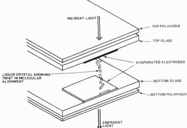
Figure 6. Operation of liquid crystal cell. Molecules of the liquid twist as shown when an electric field is set up across the cell. Under these conditions the passage of incident light becomes blocked
