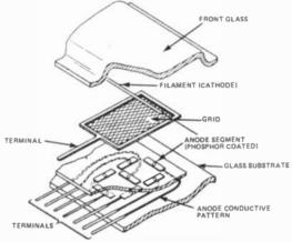
Figure 9. Typical construction of a vacuum fluorescent display (Futuba FDP)
