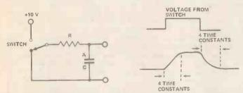
Figure 14. Circuit similar to that in Fig.13, to demonstrate effects of time-constants. Here the positions of the capacitor and resistor have been swapped
