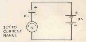
Figure 8. How to measure leakage current through an electrolytic capacitor
