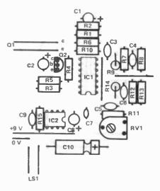
Figure 2. Overlay of the receiver PCB
