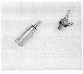
Figure 1. Phono plug (left) and socket. The socket bolts directly onto the case of the circuit.
