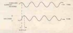
Figure 18. Waveforms of (a) current and (b) voltage for a capacitor connected to an AC supply. the peak current always occurs a quarter of a wave earlier than the peak voltage
