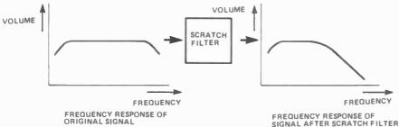
Figure 1 shows the circuit diagram of the filter, and this uses a conventional 12 dB per octave circuit (ie, above the corner frequency, doubling the frequency causes a four-fold reduction in gain).
