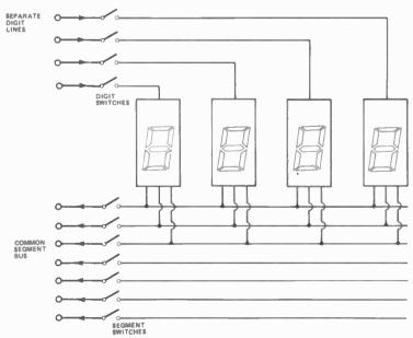
Figure 3. How the segments of a four-digit display are multiplexed. In practice all the switches are electronic end are contained within a single integrated circuit (multiplexing IC)
