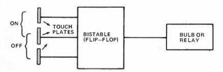
The full circuit diagram is shown in Fig.1 on page 51 of last month's HE. When power is first applied, the circuit takes up a state where transistor Q1 is biased into conduction by way of the load and resistor R1. This gives practically O V at the drain terminal of Q1, and transistor Q2 is therefore cut off as it receives no significant bias voltage via resistor R4. Both transistors are VMOS types and are therefore voltage operated - unlike ordinary bipolar devices which are current operated.
