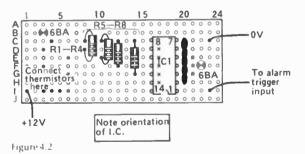
Layout of the circuit board for the fire alarm, on the underside of the board cut strips at C4, D17, E17, F17, G17, 117, Inot C17, H17) E21, F21, G21 Solder blobs join six strips: C20 to D20 to E20 to F20 to G20 to H20
