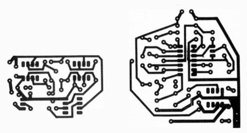
The PCB foil pattern for the Sound Torch Transmitter (left) and Receiver
