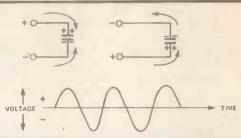
Figure 17. Effect of AC — the capacitor alternately charges and discharges for each direction of voltage, so that current flows continually
