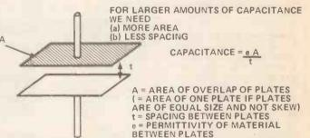
Figure 2. Parallel-plate capacitor, and the equation for capacitance
