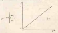
Figure 3. Capacitance, charge and voltage. Connecting a capacitor to a voltage results in a quantity of charge to be stored in the capacitor, and a graph of the amount of charge plotted against voltage is a straight line
