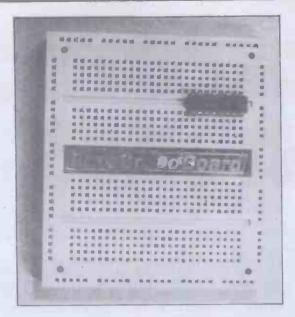
Figure 2. Using Eurobreadboard along with an integrated circuit. The holes of the Eurobreadboard are arranged so that an IC can be plugged in as easily as any other component
