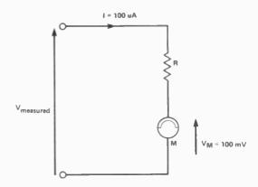
Figure 2. A series resistor added to your meter allows it to indicate higher voltages
