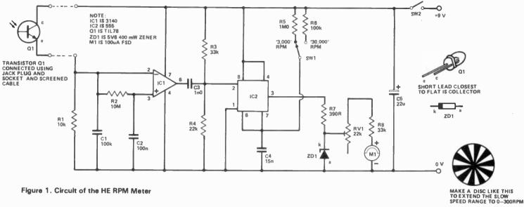
Figure 1. Circuit of the HE RPM Meter
