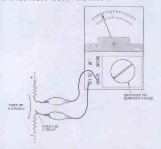
Figure 7. Making a current reading. The circuit is broken and the meter is connected into the break so that the current flows through the meter
