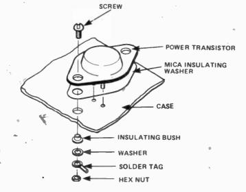
Figure 5. How to fasten transistor Q2 onto the case. If you have any, smear a small amount of heatsink compound onto both sides of the insulating washer to aid heat conduction
