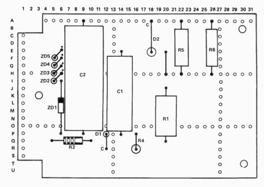
Figure 6. Veroboard layout of the project.
