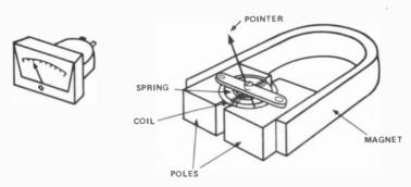
Figure 1. Typical external appearance and internal construction of a moving-coil meter
