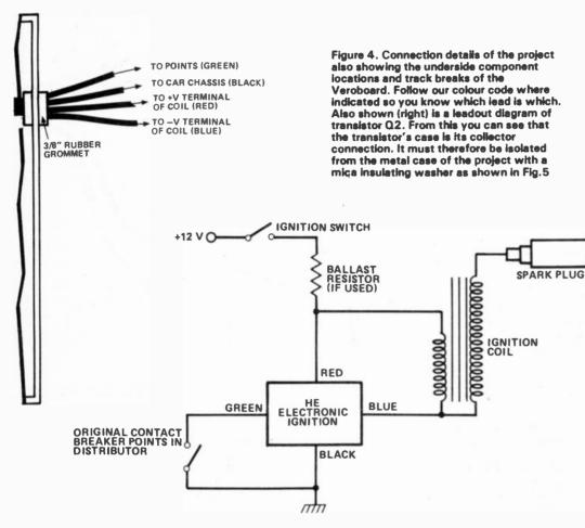
Figure 7. How the HE Electronic ignition fits into the standard Kettering ignition circuit. The lead colours shown are those adopted in Fig.4. If you use a different colour code when wiring up your project simply change the suggested colours in this diagram to your own
