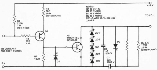
Figure 1. Circuit of the HE Electronic ignition project
