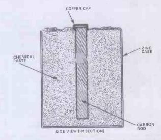
Figure 4. Conventional zinc-carbon cell, which is the unit used for most batteries
