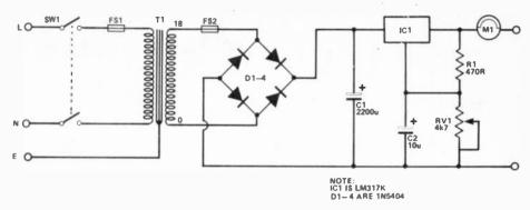
Figure 2. Circuit of the HE Variable Bench Power Supply — it's very simple, because the complicated things happen inside IC1  $\,$
