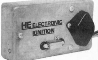
Ready for use — the HE Electronic Ignition project (see page 10) which when complete requires only four connections to your car's Ignition system. (The project shown on this month's cover was the prototype, with its high-power resistor mounted in the case. The final version has a surface-mounted resistor as shown above, for better heat dissipation
