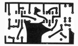
PCB foil pattern of the HE RPM Meter
