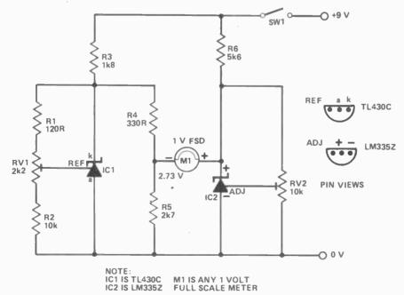
Figure 1. Circuit of the HE Thermometer
