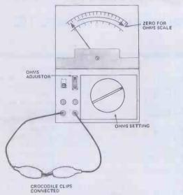
Figure 9. Making a resistance reading using one of the ohms scales of the HE Multitester: a) join the crop clips together and adjust the ohms adjustor until the needle points to zero (0) on the ohms scale, b) connect the clips to each lead of the resistor under test, as shown. A similar procedure is used with other meters. with the exception of a few from Russia
