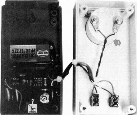
Left. Internal view of the HE RPM Meter.
