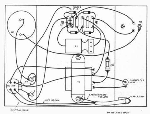
Figure 3. Wiring and connection details of the project
