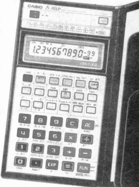
allow full register arithmetic plus display/register exchange, and one M-register, which gives one-touch recall, but allows only M + and M - arithmetic. All seven memories are non-volatile as is program storage and calculator mode.
