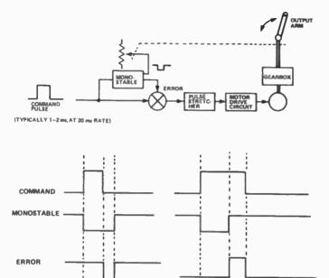
Figure 1. Remote control, by means of digital pulses, of a servo system
