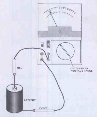
Figure 6. Making a voltage reading with a meter. The probes are connected to the points across which the voltage is to be read
