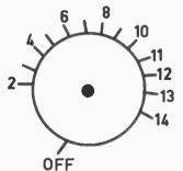
Figure 4. Mark the front panel control with this scale to give an accurate indication of output voltage
