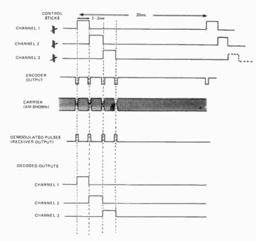
Figure 2. Waveforms associated with encoding and decoding of control signals for a three-channel system
