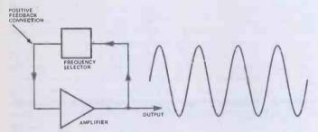
Figure 2. Block diagram of an oscillator
