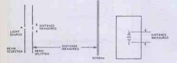
Figure 2. The method Hertz used to measure wavelength of light: (a) a slit in an opaque sheet selects one ray of light, which is then split into two by close-spaced splits in another sheet. The image projected on the screen (b), when examined with a microscope, consists of alternate dark and light bands caused by wave interference. The wavelength can be calculated from the distances indicated
