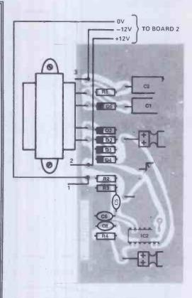
Figure 3. The edge of Board 1 where power connections are taken to Board 2
