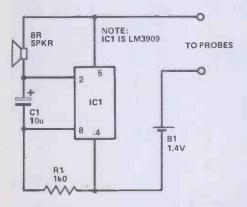
Figure 1. Circuit of the **Continuity Checker**
