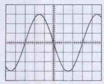
Figure 7. Example of sinewave signal displayed on typical oscilloscope screen. Timebase has been set to 5 ms/cm and vertical attenuator to 1 V/cm
