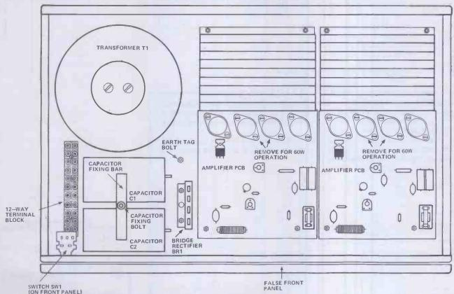
Figure 1. Positioning details of the major parts within the chassis of the HE Power Amplifier
