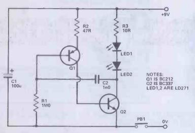
Figure 1. Circuit of the infra-red transmitter
