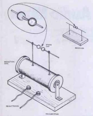
Figure 1. Hertz's transmitter and receiver. The induction coil is a DC to AC converter producing high-voltage pulses (about 40 kV)
