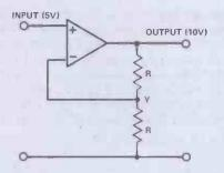
Figure 6. Op amp in non-inverting mode as a negative-feedback amplifier
