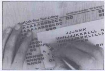
Figure 2. Transferring characters from the sheet to the front panel. Here a burnisher is shown in use
