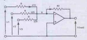
Figure 4. Op amp used as a summing amplifier
