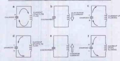
Figure 11. A charged capacitor in a resonant circuit. Figures 11a to 11f show how the charge produces a current which then charges the capacitor in the opposite direction, reversing the current until the charge is almost at its original value
