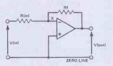
Figure 3. Circuit arrangement to show that voltage  $A_{\nu}$  is equivalent to Rf/R(in)
