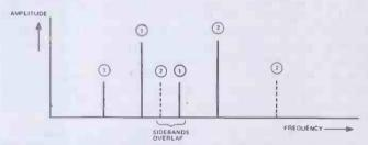
Figure 7. Interference is caused when the sidebands of two transmitters overlap, even though the carriers are separated
