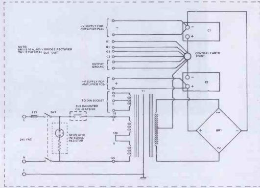
Figure 3. Circuit of the power supply used in this project
