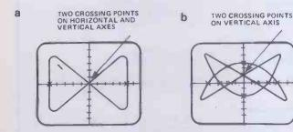
Figure 6. Lissajous figures produced by signals applied to the vertical and horizontal inputs of a 'scope: a) trace crosses horizontal axis at four points (twice at centre of screen) and vertical axis at two points (both at centre of screen), b) six crossing points on horizontal axis and four on vertical axis
