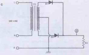
c) two-diode, full-wave rectified circuit, with resistive load.
