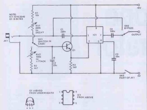
Figure 1. Circuit of HE Envelope Generator
