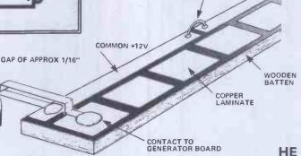
Figure 4 (above). Details of one key contact. This should be repeated along the length of the keyboard, until all 60 notes have a working contact
