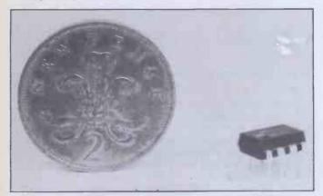
Figure 1. Comparison in size between a 741 operational amplifier and a 2p coin
