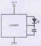
The output stage of the circuit is quite powerful and a small 8R loudspeaker can be driven directly, replacing the LED in the above circuit.
