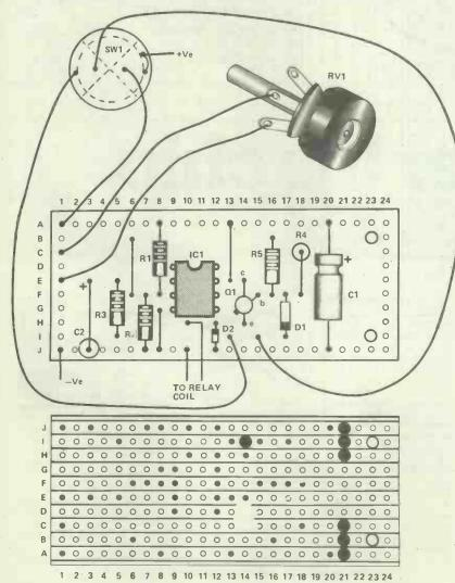
RESISTORS (All ¼ W, 5%) R1,2,5 3k9 R3 6k8 R4 47k POTENTIOMETER RV1 470k linear potentiometer CAPACITORS C1,2 100u, 10 V electrolytic SEMICONDUCTORS IC1 LF351 or TL081CP, bifet operational amplifier D1,2 1N4148, diode Q1 BC109, NPN transistor MISCELLANEOUS SW1 four-pole, three-way rotary switch RLA 12 V relay 185R, with at least one set of heavy-duty, normally-open contacts Case to suit 10 strip x 24 hole, 0.1" Veroboard Knobs
