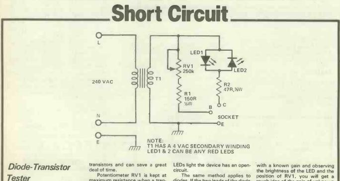
No apologies are made for including this circuit - there is nothing particularly new about it, but it is very useful when checking diodes and
