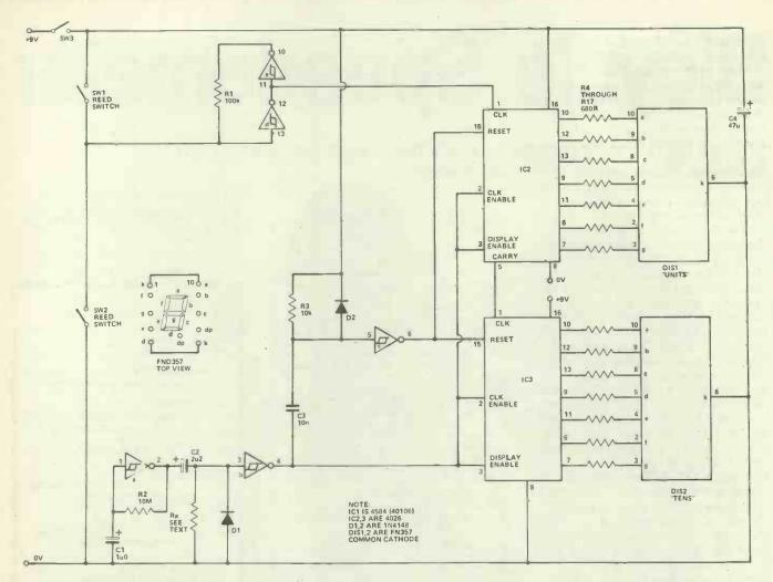
Figure 1. Circuit diagram of the HE Bicycle Speedometer
