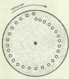
Figure 2. Nipkow disc, the scanning system used by most of the mechanical TV systems
