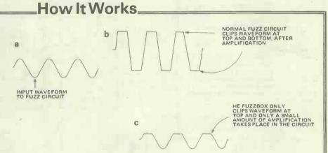
Figure 3. a) A possible input signal b) The output of a conventional fuzz circuit c) The output of the HE Fuzzbox
