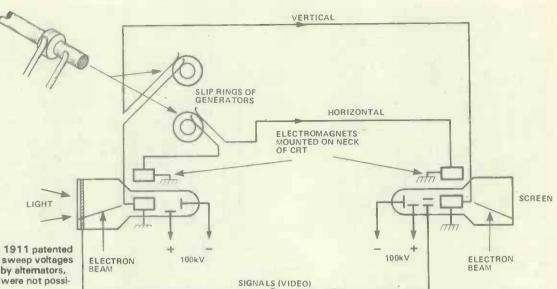
Figure 4. Campbell-Swinton's 1911 patented sketch in simplified form. The sweep voltages were to have been generated by alternators, because electronic oscillators were not possible at that time
