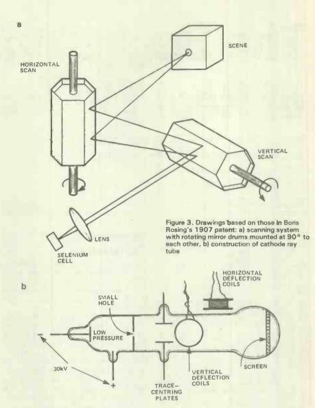
generated by passing current through a gas at low pressure rather than by thermionic emission, the deflection system and fluorescent screen were virtually the same as those we would recognise today. The possibilities which were opened up by this invention were immediately recognised by research physicists, who seized on the new device as a method of displaying alternating voltages. Engineers took a bit longer to see what might be achieved.
