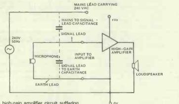
Figure 4. A high-gain amplifier circuit suffering from capacitive pickup
