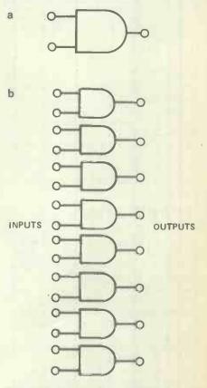
Figure 7.1 One operation — ANDing, A single AND gate (a) can AND two bits. To AND a set of eight bits (b) would need eight AND gates, with sixteen inputs and eight outputs
