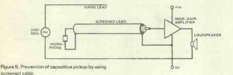
sulator. So between our two amplifier leads and also between the signal lead and the mains lead in Fig. 4, capacitances exist and are indicated by capacitor symbols. These two capacitors form a potential divider and a small part of the mains voltage is superimposed on the signal lead. The amplifier, as you would expect, amplifies this with the result that a 50 cycle-per-second (Hz) 'hum' is heard from the loudspeaker. This frequent problem is called 'mains hum'.
