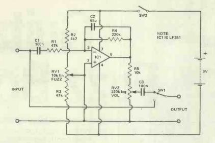
Figure 1. HE Fuzzbox circuit diagram. The simplicity of the project makes it ideal for the beginner
